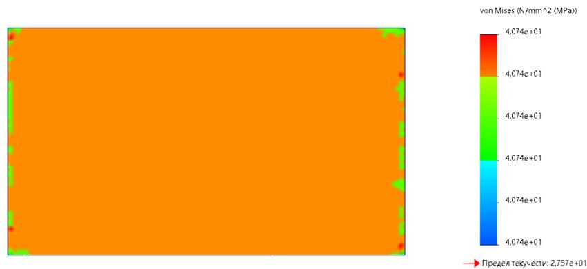
Fig. 5. Stress distribution in the solid foil at standard mesh resolution.
