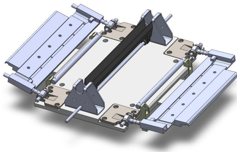
Fig. 3. Initial assembly model of the device.
