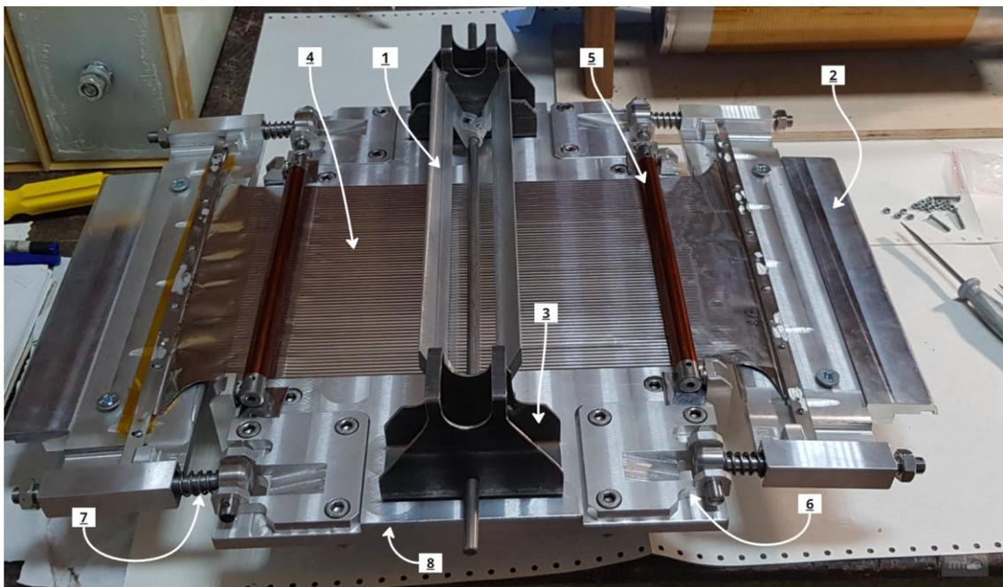
Fig. 1. Foil tensioning device
