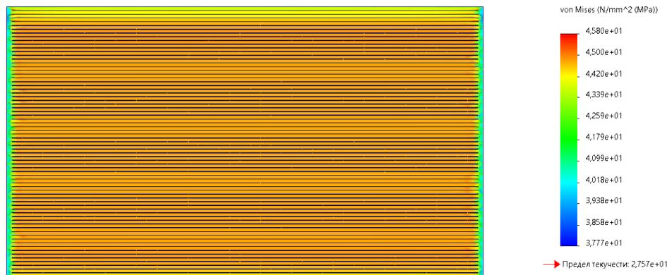
Fig. 6. Stress distribution in the foil with strips at standard mesh resolution.
