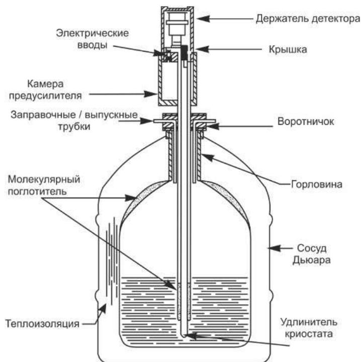
Figure 1. Appearance and design of detection units in a vertical submersible cryostat with nitrogen cooling.
