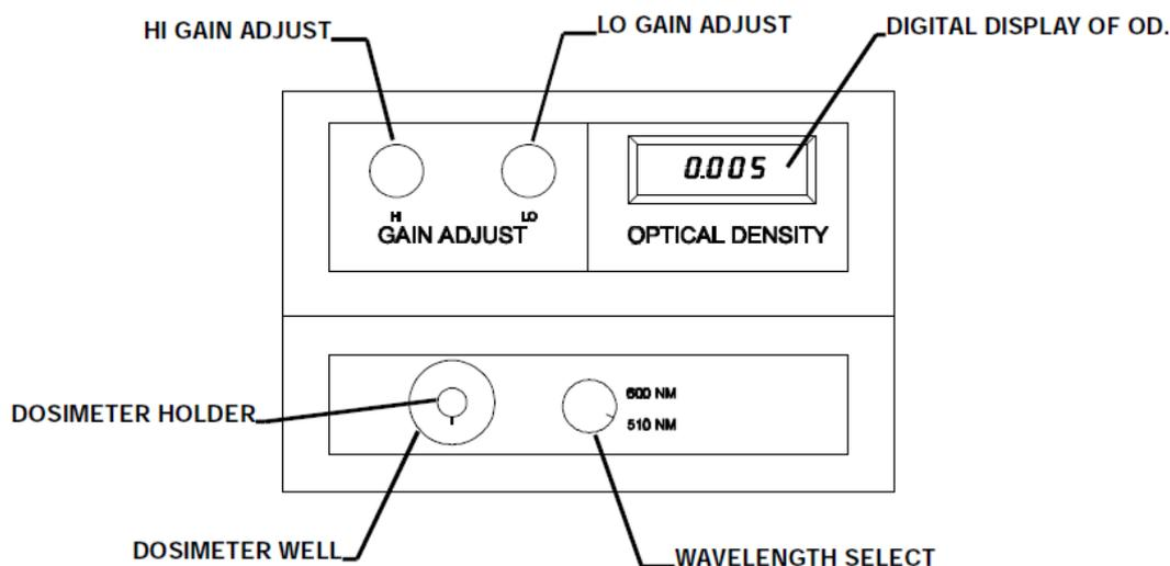
Figure 3. The appearance and basic controls of the FWT-92 photometer.
