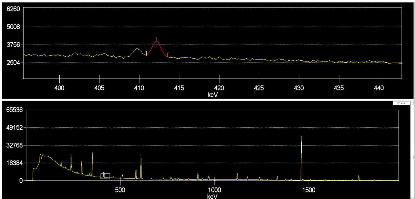
Figure 6. The spectrum obtained after irradiation of the gold indicator (bottom), the gold line on an enlarged scale (top).
