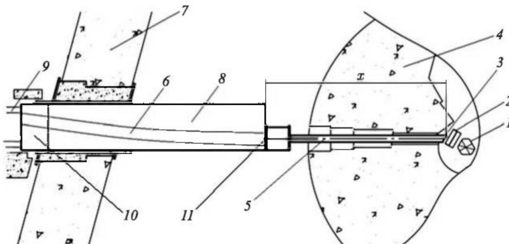
Figure 4. Experimental setup for radiation research on the IBR-2 beam No. 3 [9]: 1 — IBR-2 core; 2 — Water moderator — WM-303; 3 — end of the straight section (I-beam) for the installation of test samples; 4 — first biological shield; 5 — straight section ( $x = 3$  m); 6 — curved section (pipe 4,87 meters long); 7 — second biological shield; 8 — steel cylinder with water; 9 — rail track; 10 — gate; 11 — initial point of the curved pipe.
