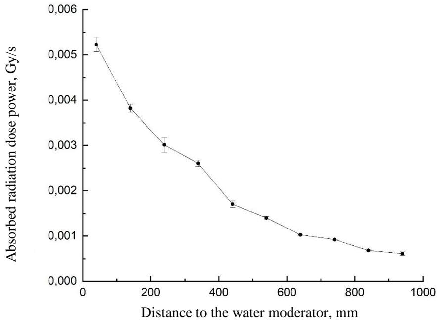
Figure 5. The dependence of the absorbed dose of gamma radiation on the distance to the WM at reactor power of  $\langle W \rangle = 0$  кВт.
