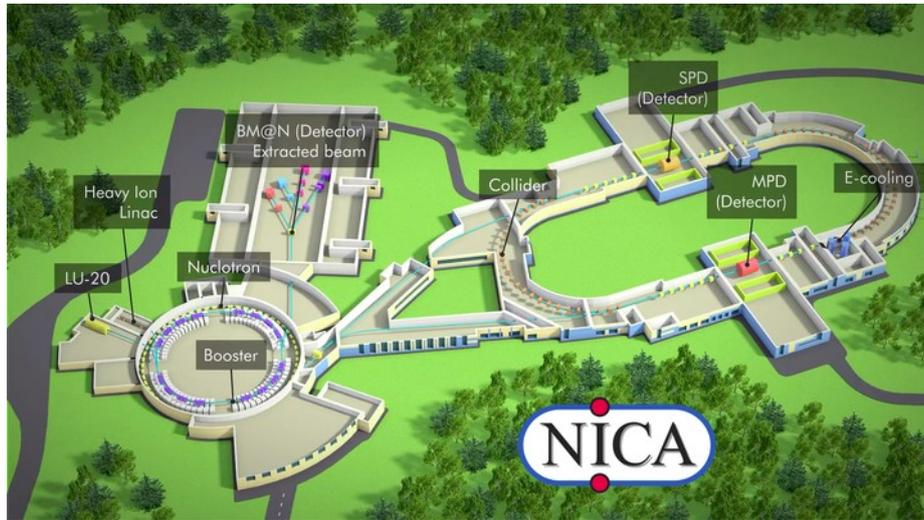
Fig. 1 - NICA complex schematic layout
