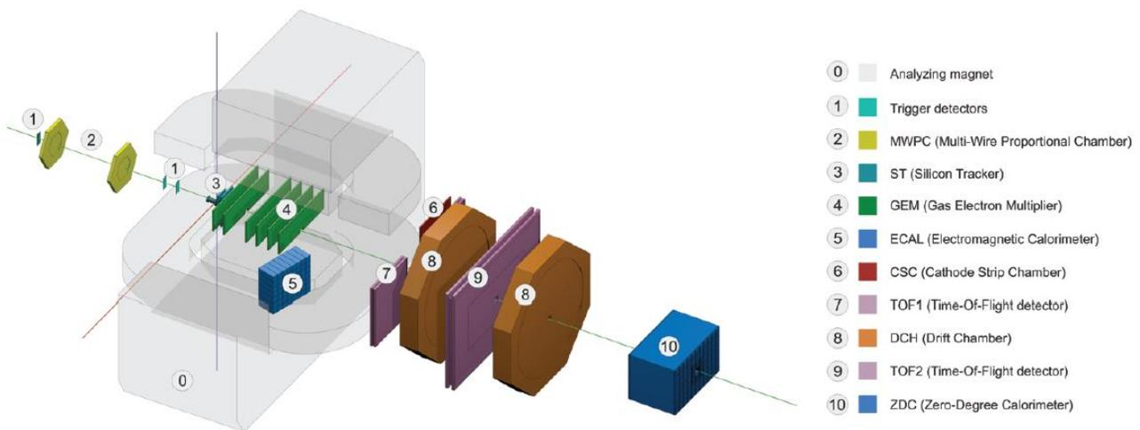
Figure 1: BM@N experimental set-up.<sup>5</sup>
