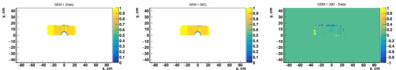
*Figure 10:* **Left:** 2-D histogram of the efficiency of the first GEM station for the real experimental reconstructed tracks. **Center:** 2-D histogram of the efficiency of the first GEM station for the MC simulated tracks. **Right:** 2-D histogram of the difference of the two efficiencies of the first GEM station.
