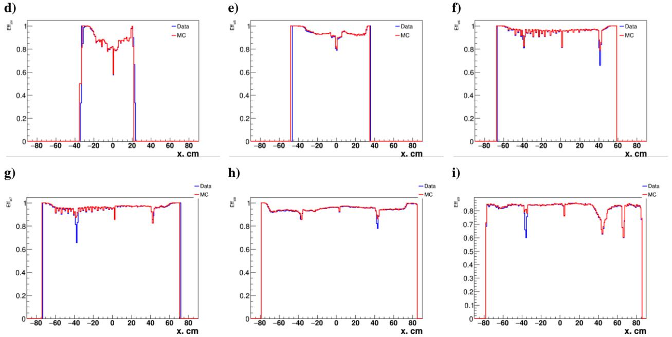
**Figure 13:** A comparison between the x-projection of the efficiencies for real experimental data (blue line) and the MC simulated data (red line) for negative tracks after three iterations for: **a)** the first FwdSi station, **b)** the second FwdSi station, **c)** the third FwdSi station, **d)** the first GEM station, **e)** the second GEM station, **f)** the third GEM station, **g)** the fourth GEM station, **h)** the fifth GEM station, **i)** the sixth GEM station.
