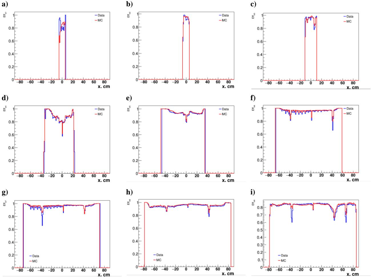
*Figure 12:* A comparison between the x-projection of the efficiencies for real experimental data (blue line) and the MC simulated data (red line) for negative tracks before additional adjustments for: **a)** the first FwdSi station, **b)** the second FwdSi station, **c)** the third FwdSi station, **d)** the first GEM station, **e)** the second GEM station, **f)** the third GEM station, **g)** the fourth GEM station, **h)** the fifth GEM station, **i)** the sixth GEM station.
