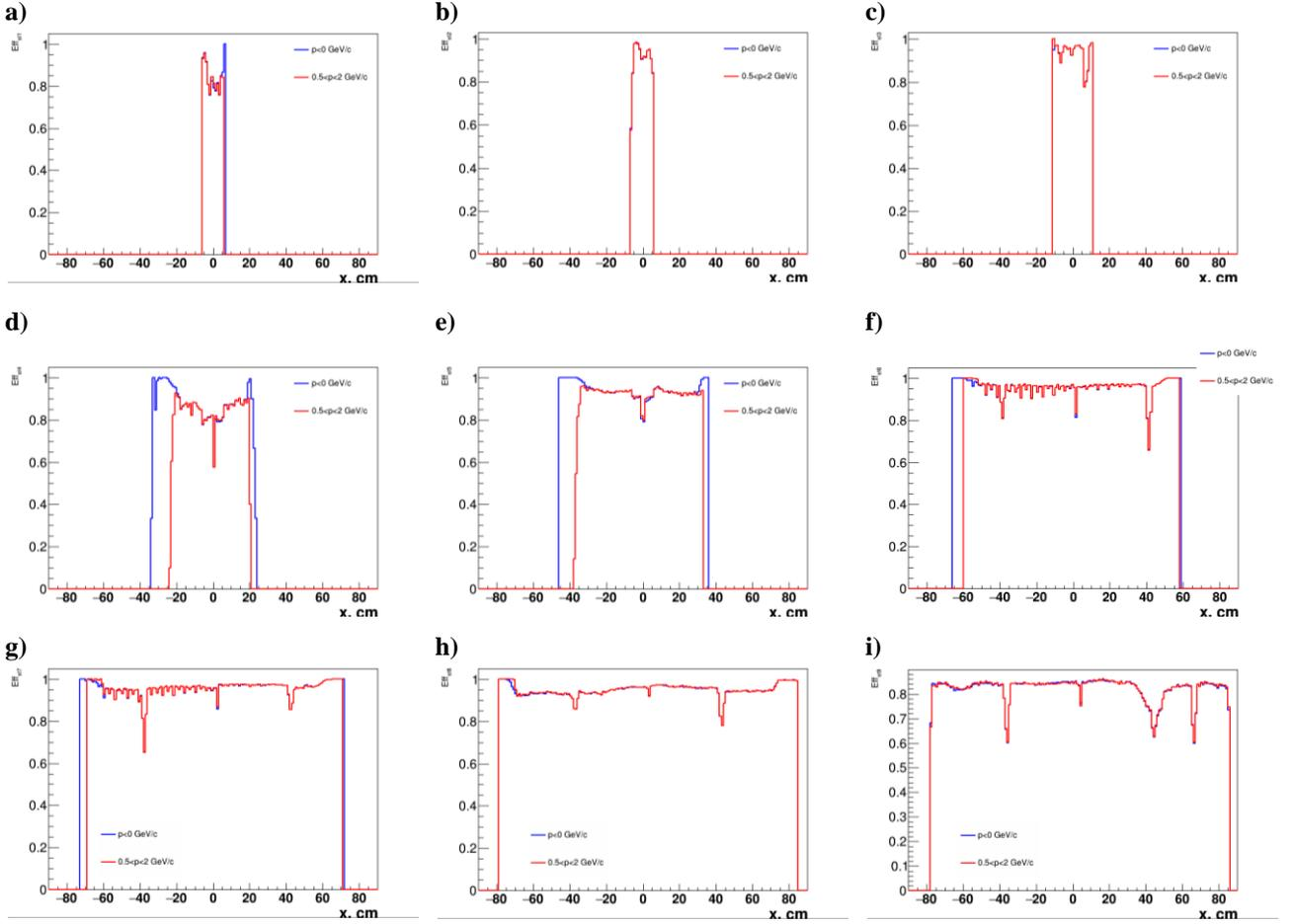
**Figure 9:** A comparison between the x-projection of the efficiencies for the negative tracks (blue line) and the positive tracks (red line) for: **a)** the first FwdSi station, **b)** the second FwdSi station, **c)** the third FwdSi station, **d)** the first GEM station, **e)** the second GEM station, **f)** the third GEM station, **g)** the fourth GEM station, **h)** the fifth GEM station, **i)** the sixth GEM station.
