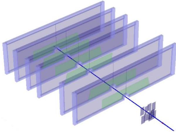
*Figure 2:* Central tracker configuration. It consists of 6 planes of GEM detector and 3 planes of FwdSi detector.
