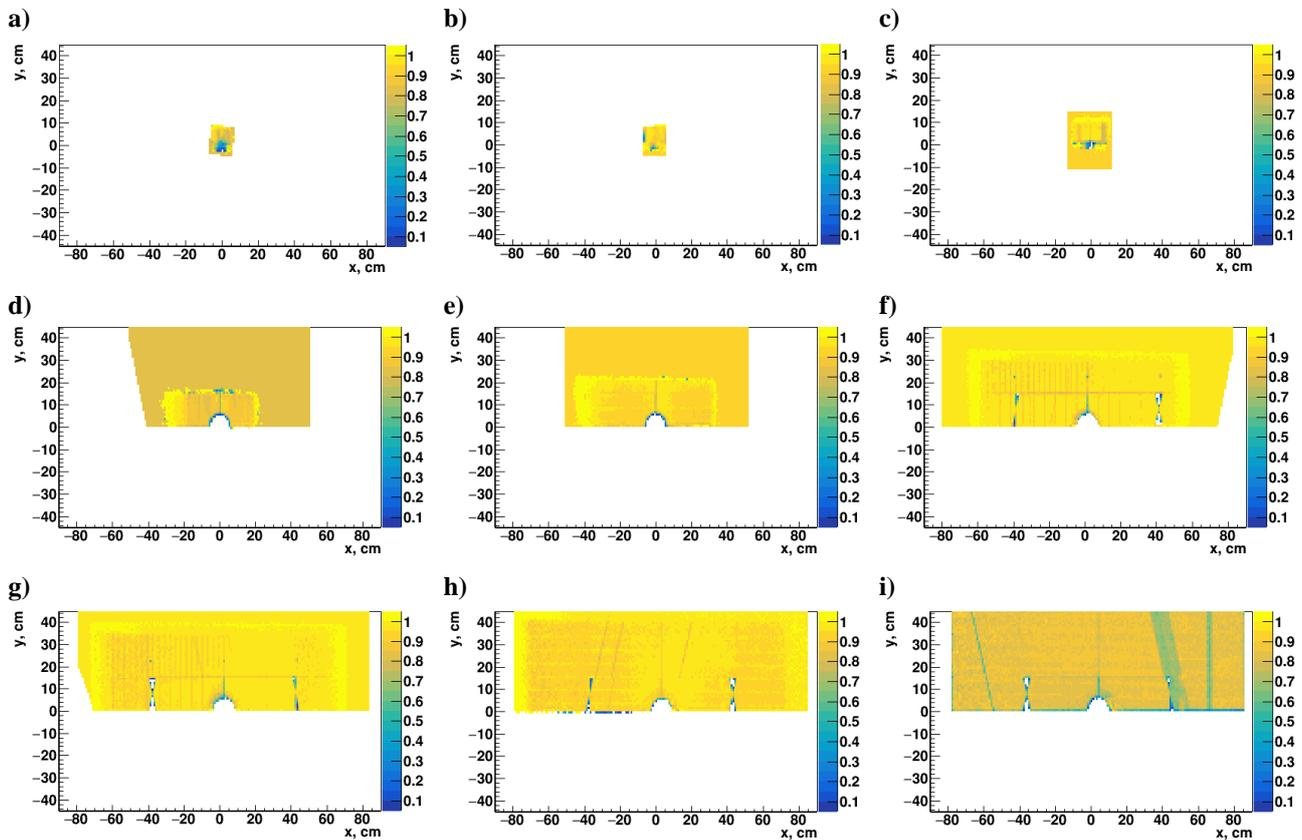
**Figure 8:** Two-dimensional efficiency histograms for negative tracks for: **a)** the first FwdSi station, **b)** the second FwdSi station, **c)** the third FwdSi station, **d)** the first GEM station, **e)** the second GEM station, **f)** the third GEM station, **g)** the fourth GEM station, **h)** the fifth GEM station, **i)** the sixth GEM station.
