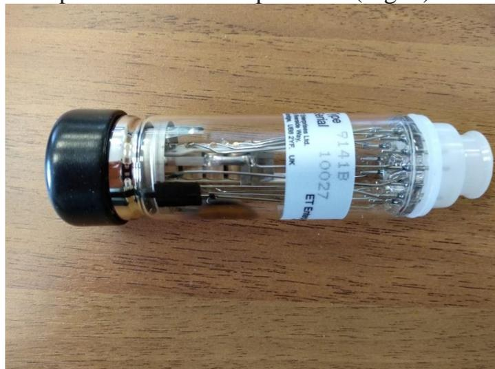
Fig. 3. The Photomultiplier ET Enterprises model 9141B
