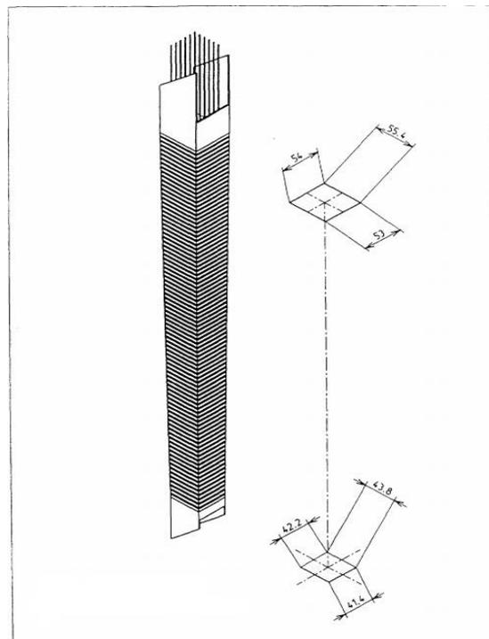
Figure B. The example shashlik tower design. View of face.
