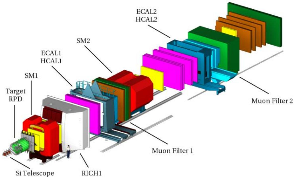
**Fig.1.** Three-dimensional view of the COMPASS setup for measurements with hadron beams. The beam comes from the left side. The upstream part of the setup (beam line) is not shown here. The different colours indicate different detector types.
