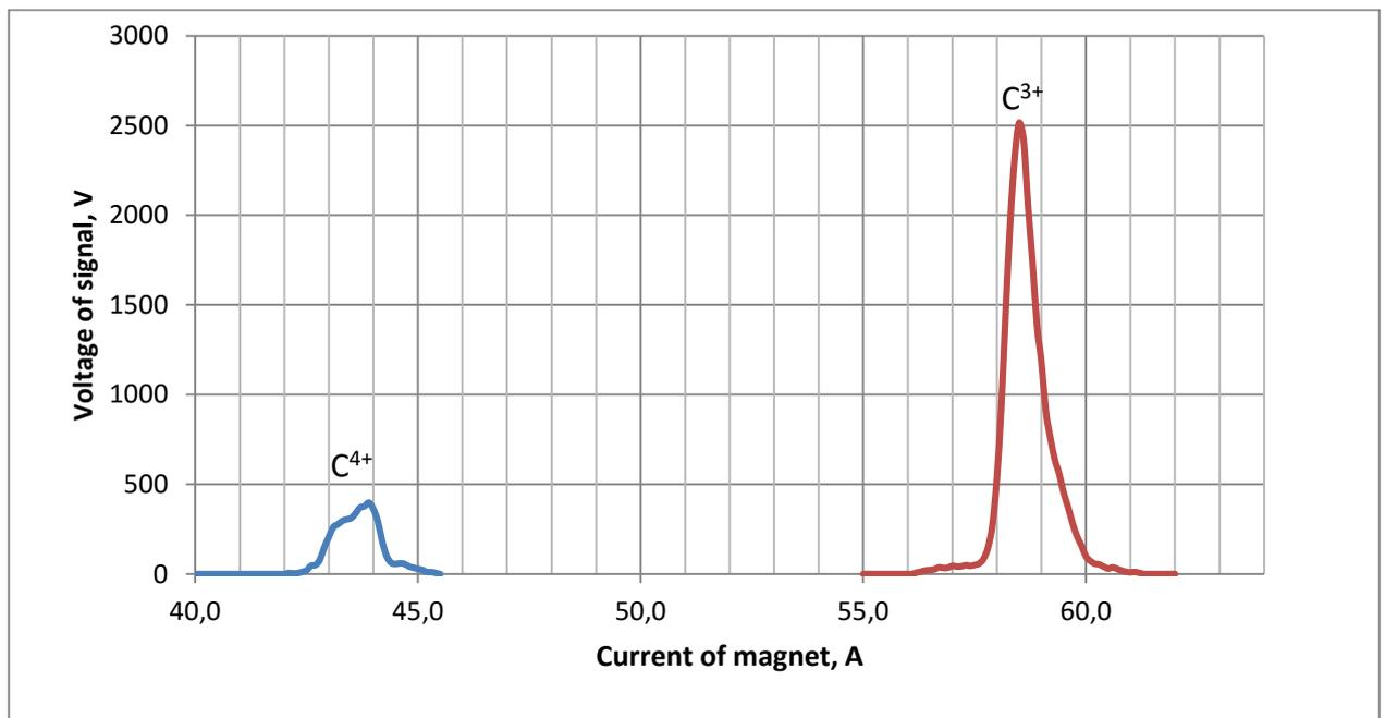
Figure 8. The spectrum of carbon ( $E_2 = 300 \text{ keV}$ )
