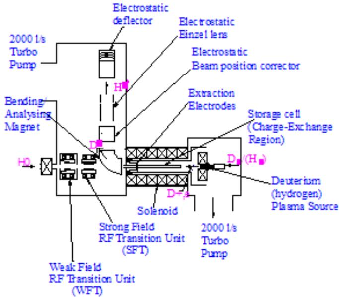
Figure 13. Schematic layout of the SPI plasma ionizer
