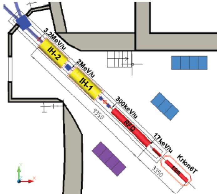
Figure 3. HILAC and its components
