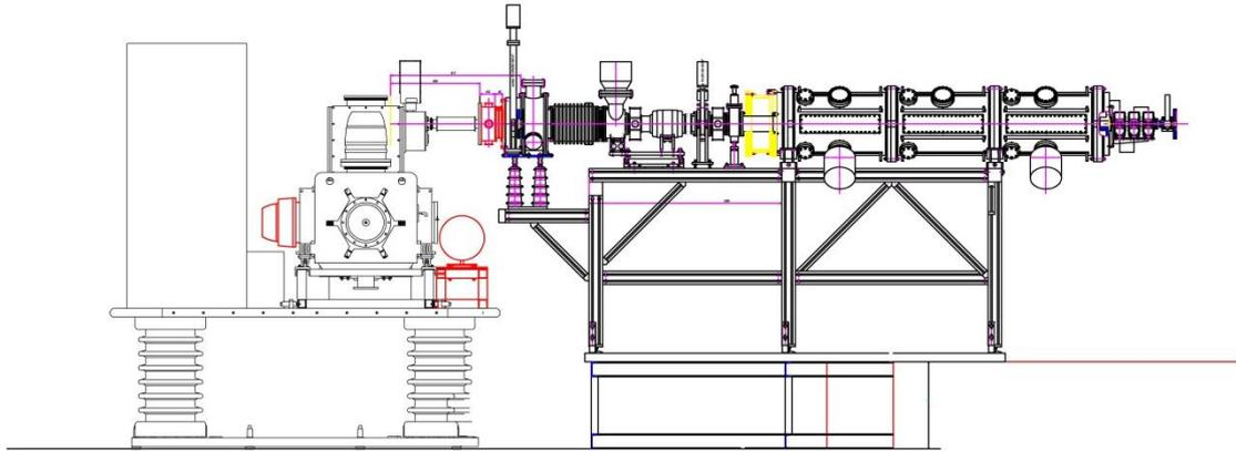
*Figure 24. Schematic layout of SPI matched with LEBT and RFQ*
