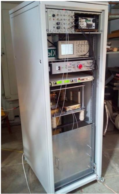
*Figure 16. High-voltage pulse generator of the arc plasma source*
