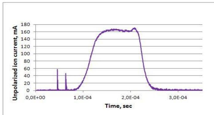
Figure 21. Unpolarized ion current (D+)
