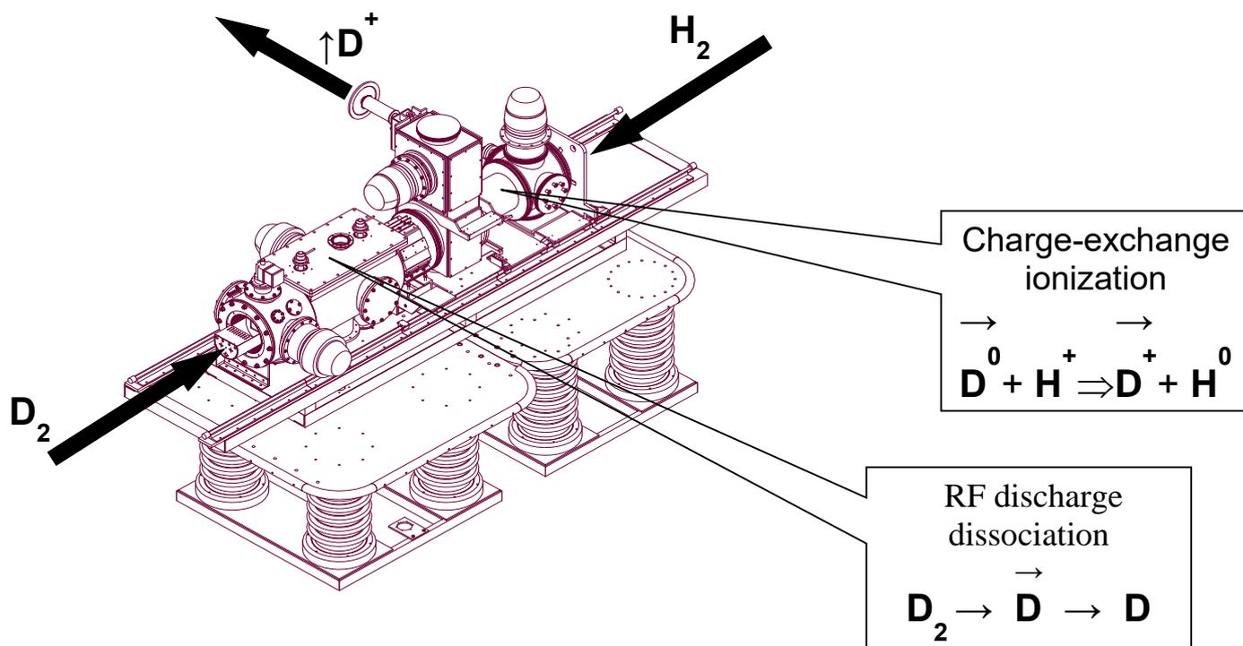
Figure 11. General view of SPI source with specifications of basic processes
