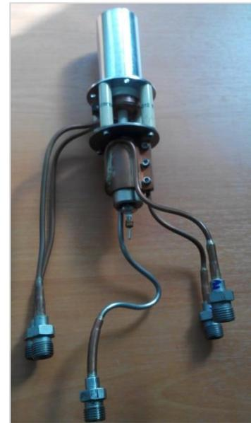
Figure 14. Hydrogen plasma source
