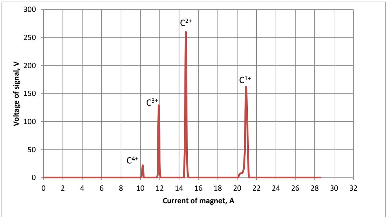
Figure 6. The spectrum of carbon ( $E_1 = 51 \text{ keV}$ )
