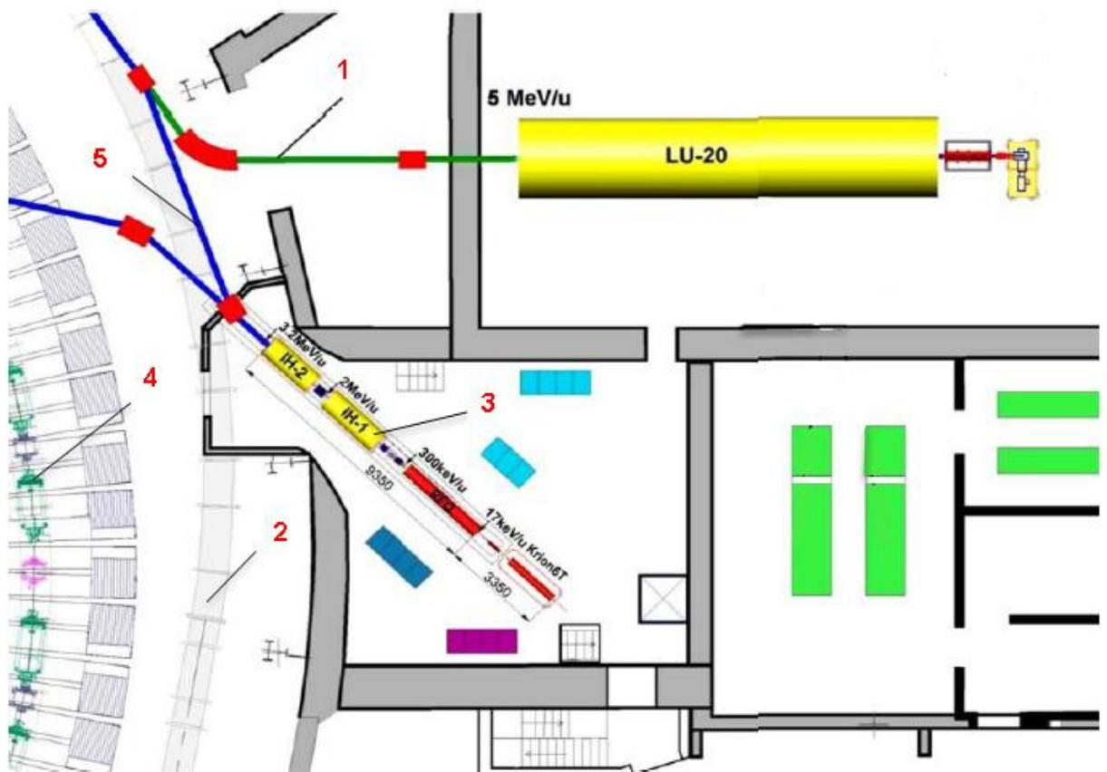
*Figure 1. Injection facility: 1 – LU-20 injection; 2 – NUCLOTRON; 3 – HILAC; 4 – Booster ring; 5 – Transport channel.*
