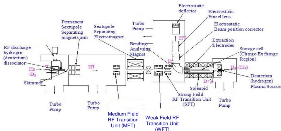
Figure 10. Schematic layout of the SPI source
