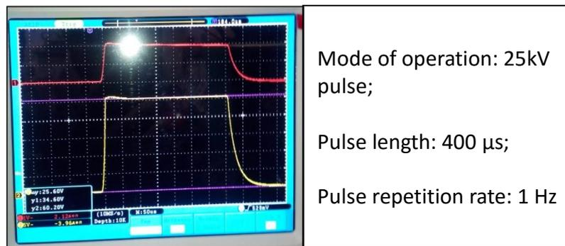
Figure 15. Hydrogen plasma source HV pulse generator
