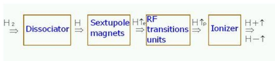
Figure 9. Process of polarized ions production in the SPI
