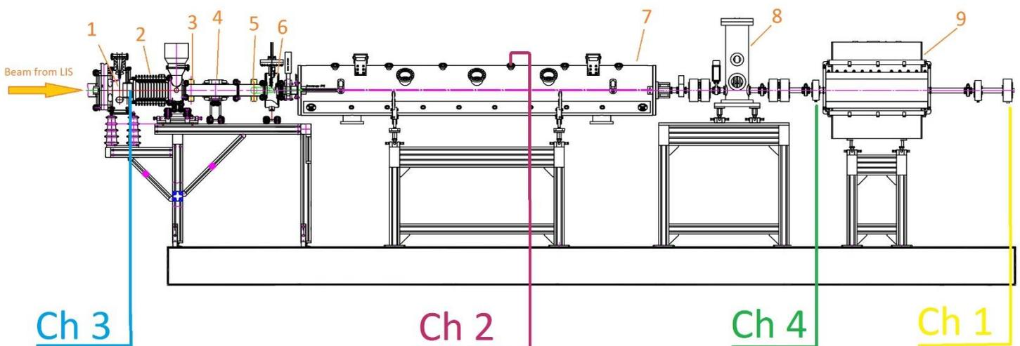
Figure 5. Schematic layout of the experiment: 1 – Electrostatic lenses (E1 and E2); 2 – Electrostatic pre-accelerator; 3 – Magnetic lens L1; 4 – Corrector; 5 – Magnetic lens L2; 6 – Faraday cup; 7 – RFQ module; 8 – Buncher; 9 – Magnetic analyzer;
