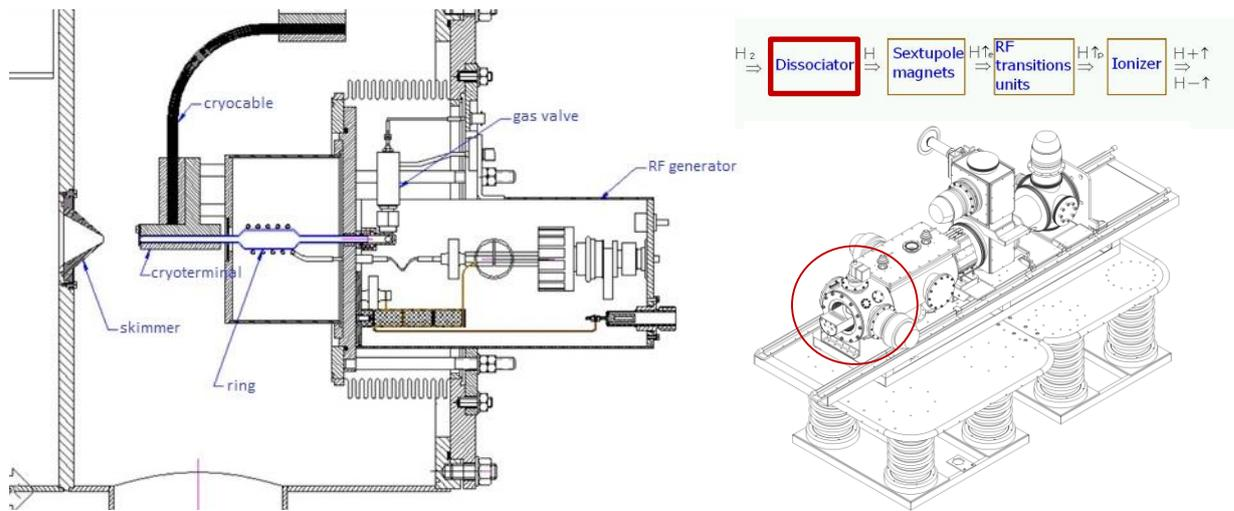
*Figure 12. Schematic layout of RF dissociator with specification of its location*
