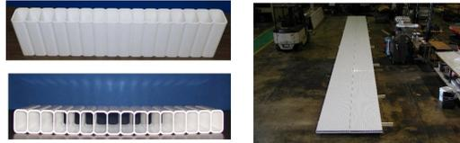
Figure 7: (a) Close-up photos of one 16-cell PVC extrusion, 15 cm long. (b) Two full-size 16-cell extrusions 15.5 m long placed side-by-side form the basis for an extrusion module.
