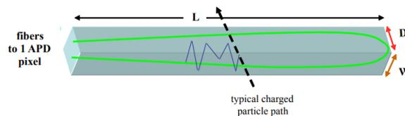
Figure 6: Schematic illustration of a PVC cell of dimensions  $W \times D \times L$  containing liquid scintillator and a wavelength-shifting fiber (green). A charged particle incident on the cell produces scintillation photons (blue line) that bounce off the cell walls until absorbed by the fiber or lost.
