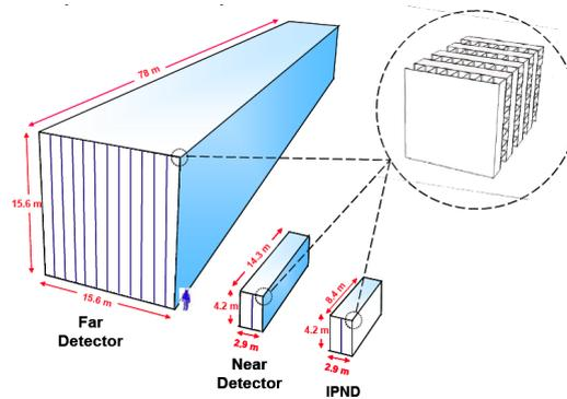
Figure 8: The far and near detector. The far detector is the largest free-standing man-made plastic structure in the world.
