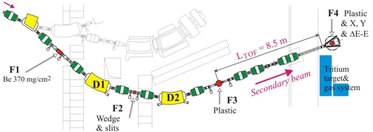
**Figure 3.** ACCULINNA *in-flight* fragment separator scheme (FLNR, Dubna) [5]
