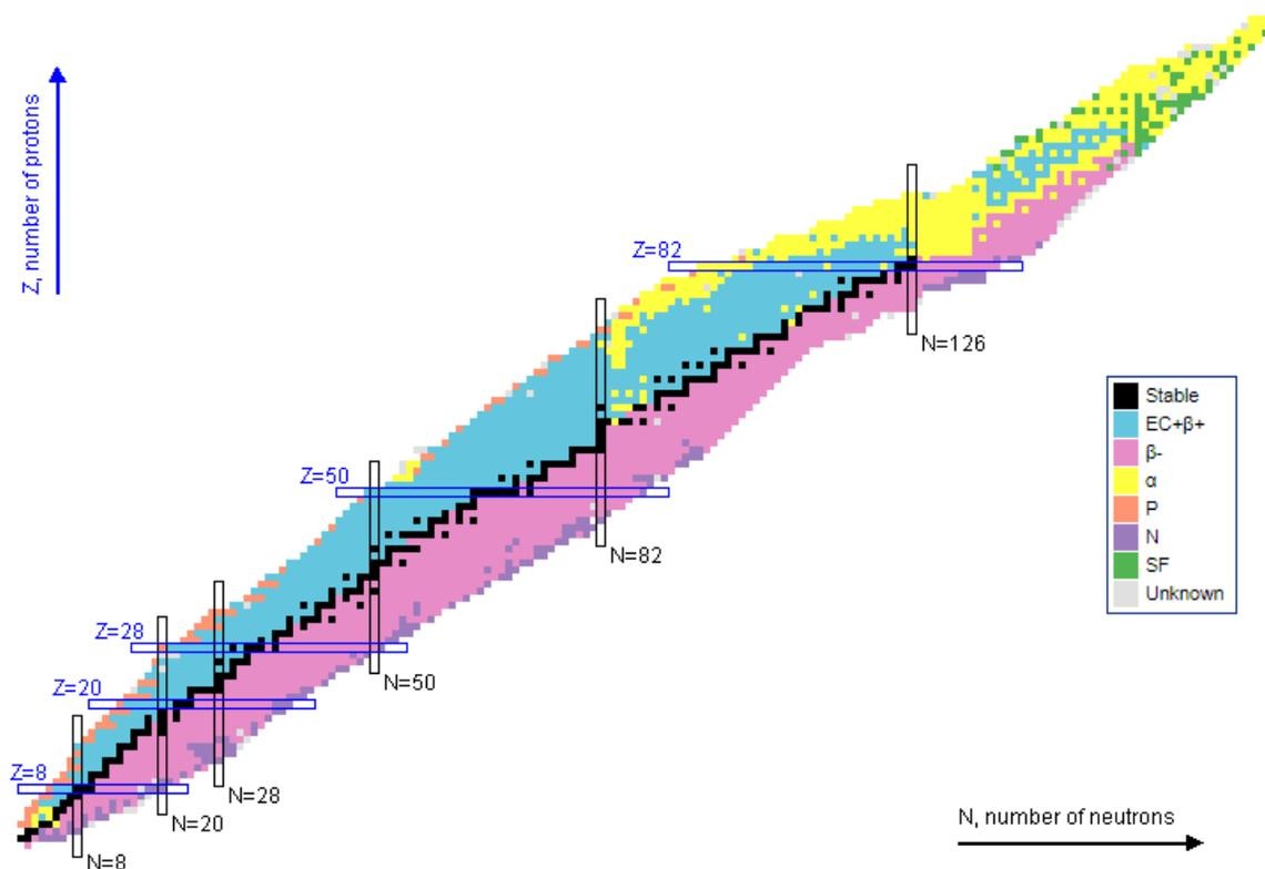
**Figure 1.** Chart of nuclides taking into account all existing decay channels [1]
