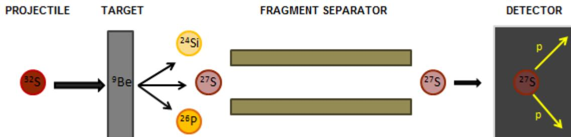
**Figure 2.** All stages of the experiment with exotic nuclei on the example of  $^{27}\text{S}$ .
