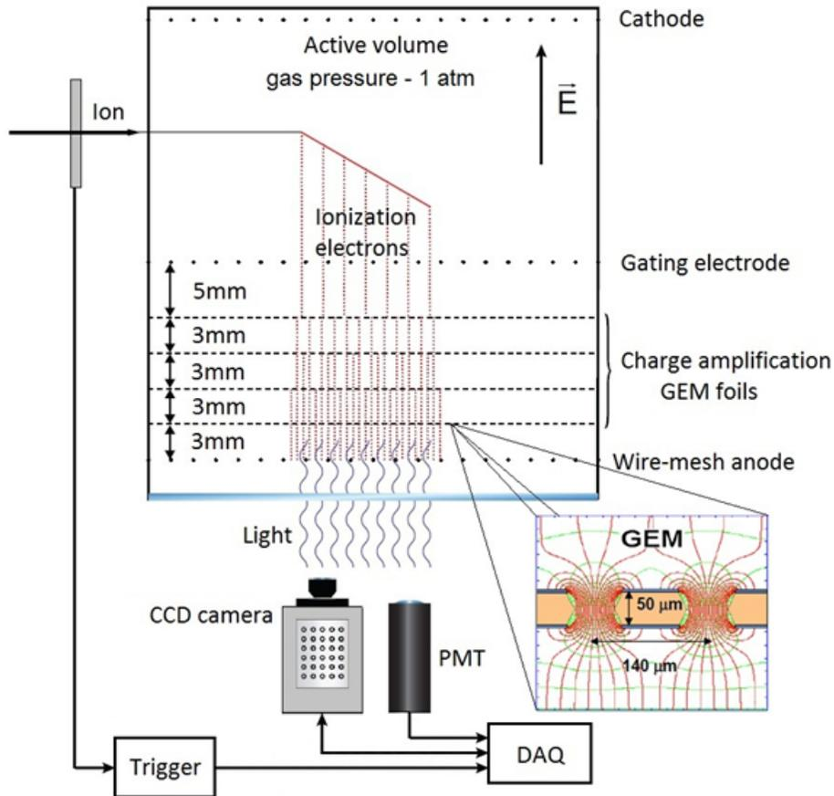
Figure 4. Scheme of Optical Time Projection Chamber [6]
