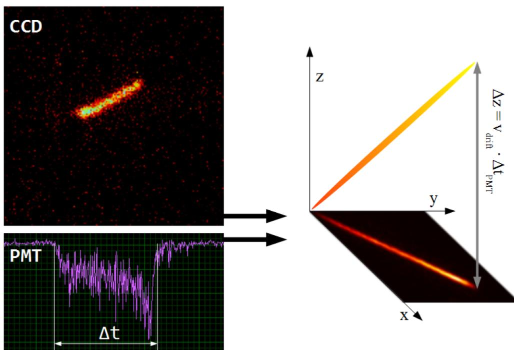
**Figure 5.** Three dimensional track reconstruction from both OTPC signals [3]
