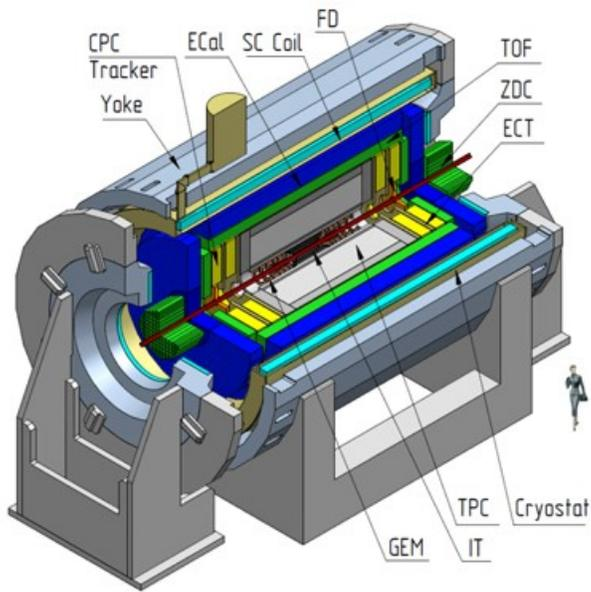
Figure 4: Multi Purpose Detector (MPD) scheme. Picture taken from [6].
