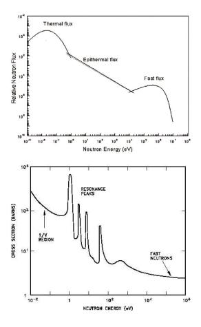
It is possible to proceed irradiation only in resonance energies by using cadmium screen. Cadmium cuts off thermal neutrons and only epithermal and fast neutrons are present. The  $E_{Cd} = 0.55$ eV value is called Cd cut off energy. The principle of neutron activation is shown on a picture below.
