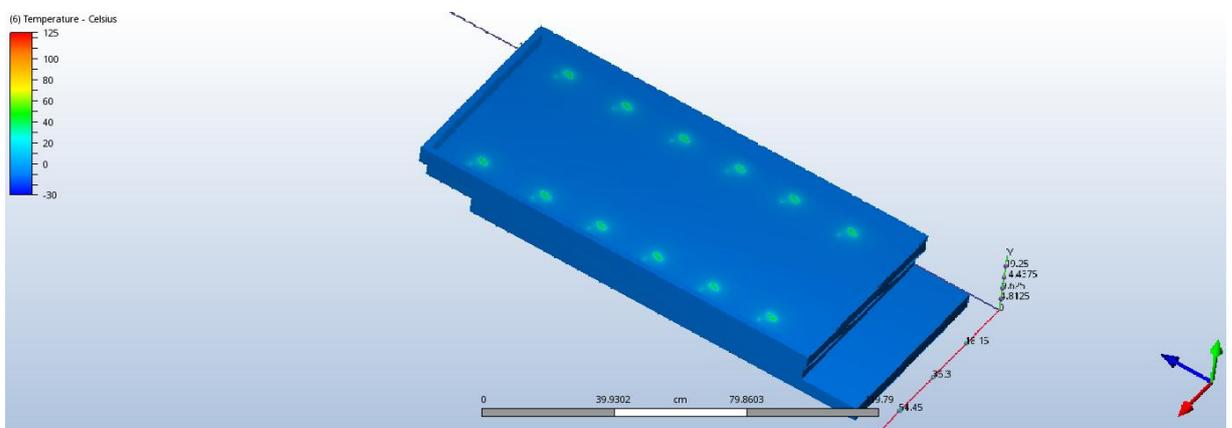
Picture 10. The MPD-TOF detector at a temperature of -10°C
