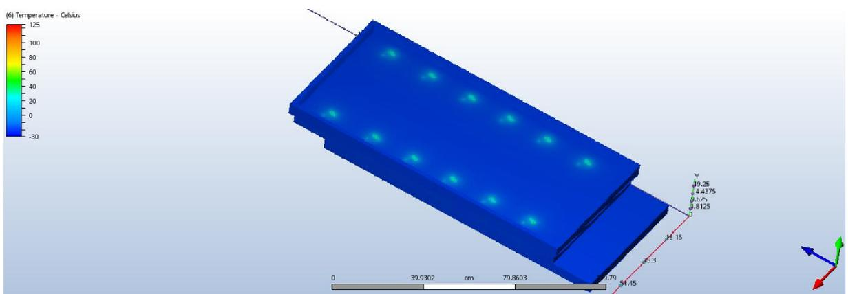
Picture 11. The MPD-TOF detector at a temperature of -20°C
