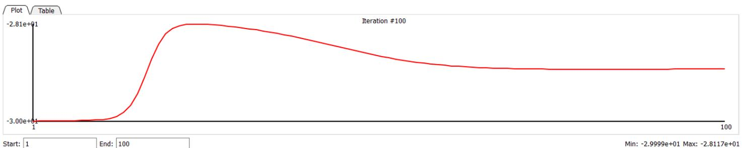
Chart 8. Temperature of complex in ambient temperature of  $-30^{\circ}\text{C}$
