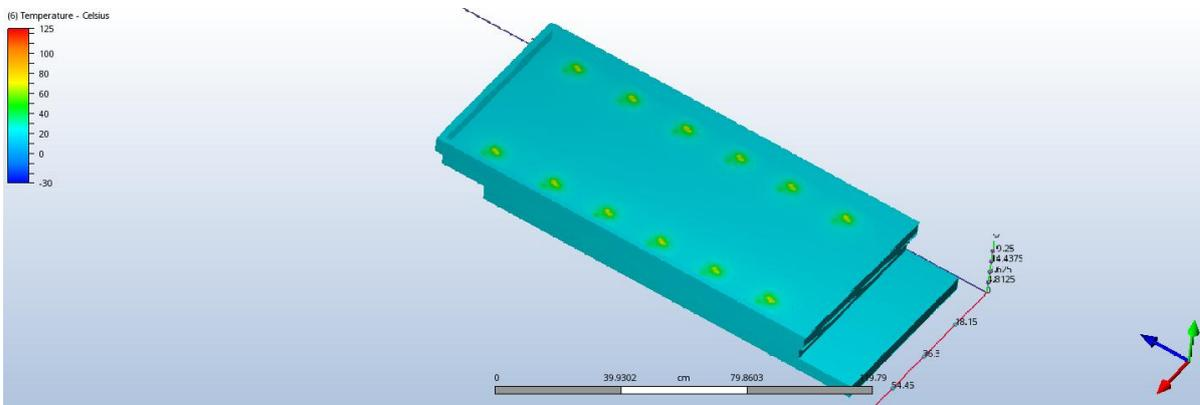
Picture 7. The MPD-TOF detector at a temperature of 20°C
