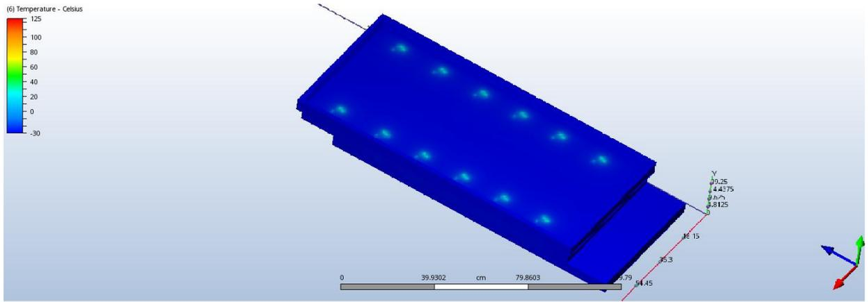
Picture 12. The MPD-TOF detector in temperature of  $-30^{\circ}\text{C}$
