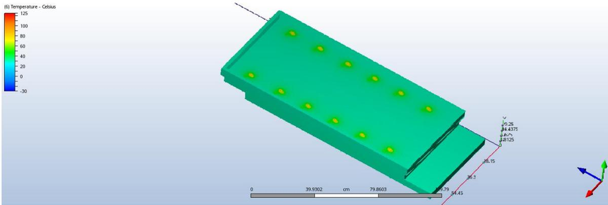
Picture 6. The MPD-TOF detector at a temperature of 30°C
