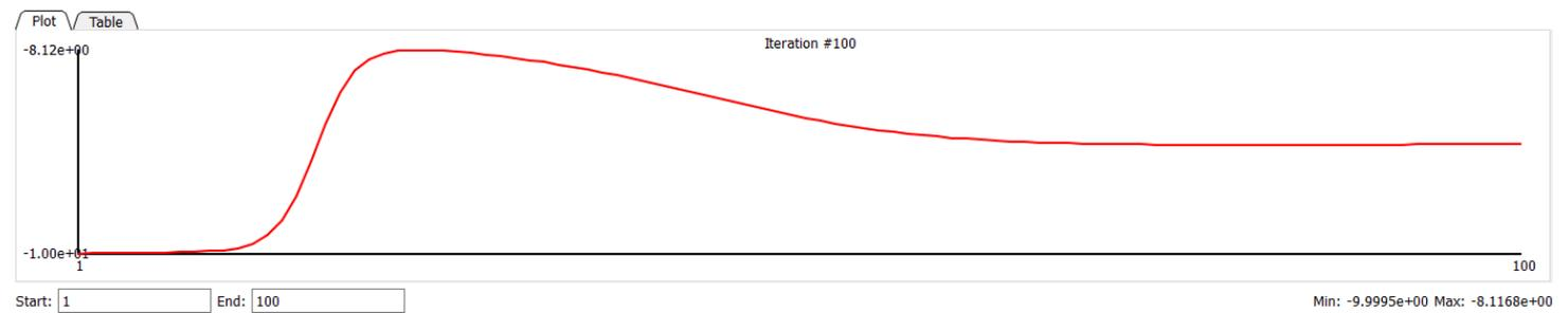
*Chart 6. Temperature of complex in ambient temperature of -10°C*
