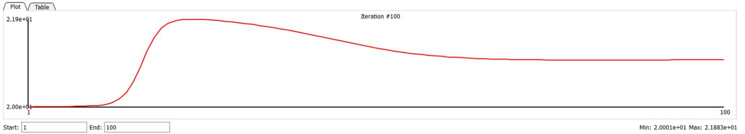
*Chart 3. Temperature of complex in ambient temperature of 20°C*
