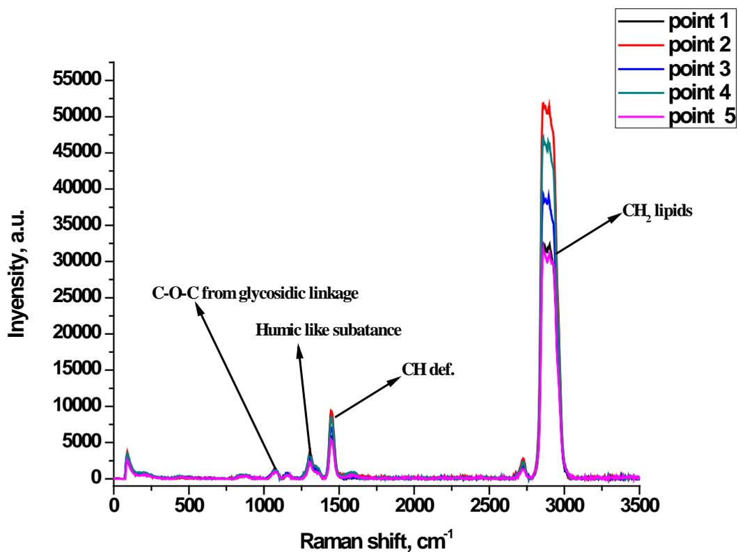
Fig (13): Raman spectrum of SRB biofilm after 22<sup>nd</sup> days (steal substrate)
