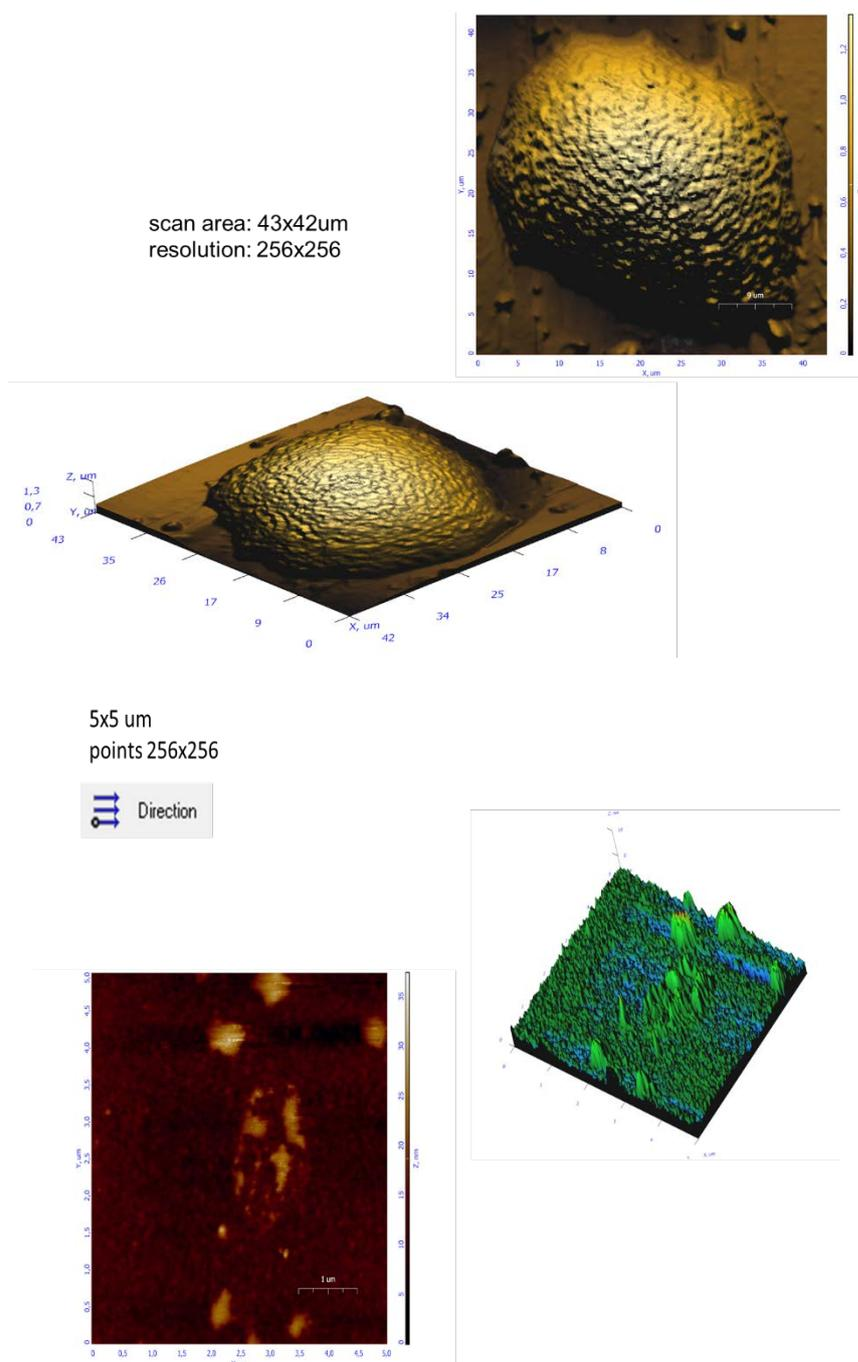
**Fig (17): AFM imaging of SRB biofilm after 10<sup>th</sup> days (steel substrate)**
