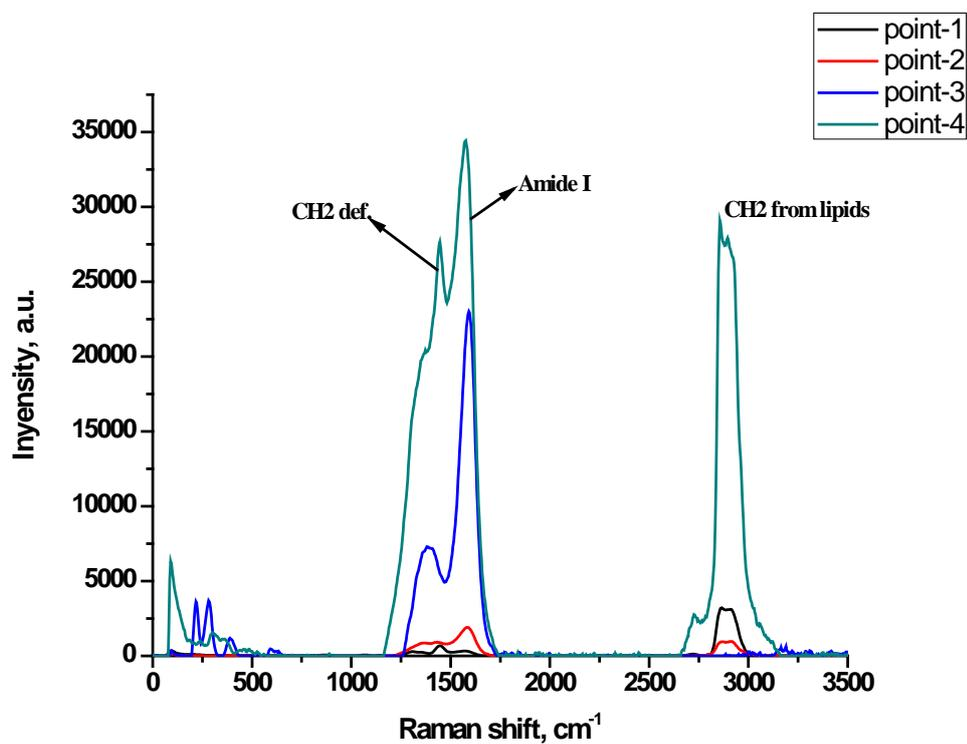
Fig (12): Raman spectrum of SRB biofilm after 15<sup>th</sup> days (steal substrate)
