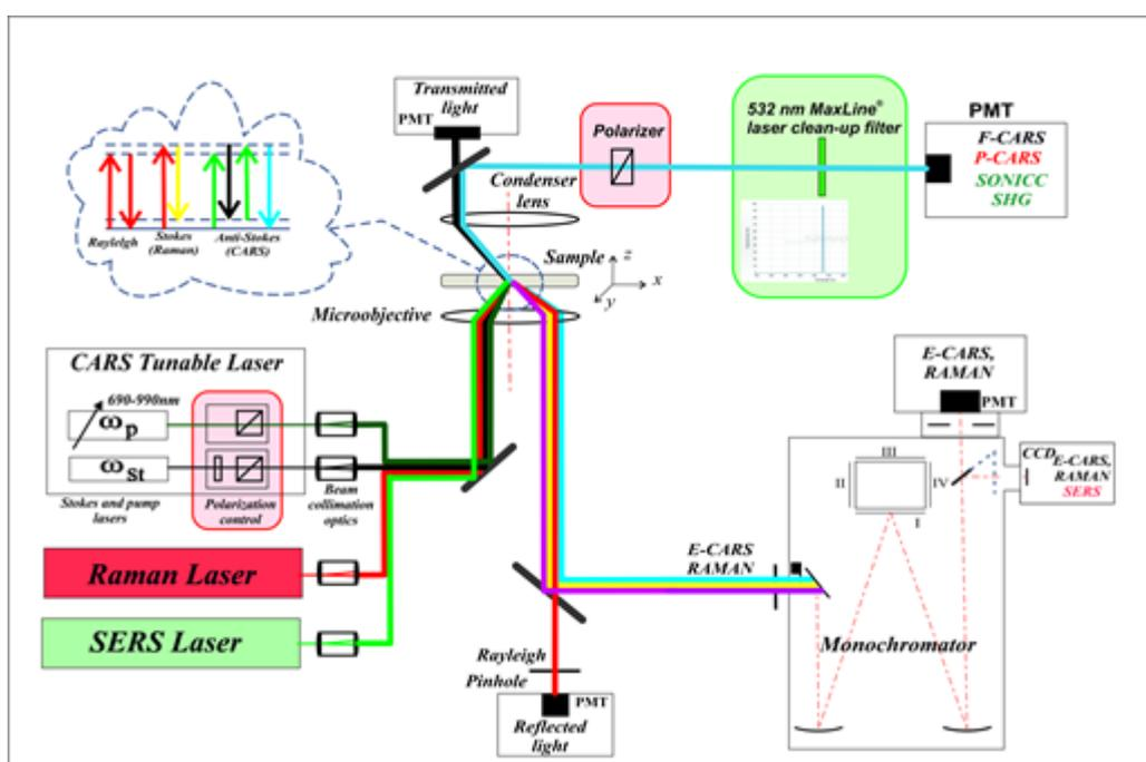
Fig (3): layout of CARS microscope.
