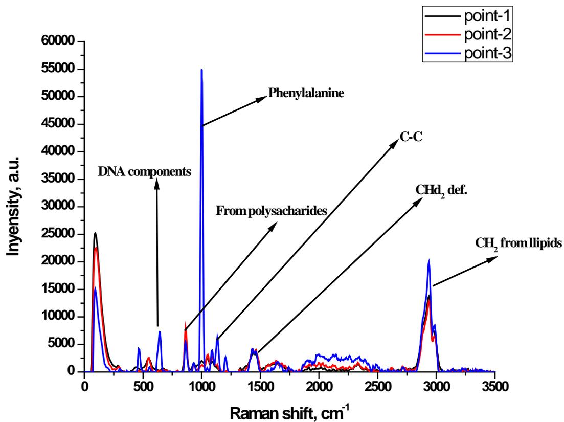
Fig (10): Raman spectrum of SRB biofilm after 10<sup>th</sup> days (scratch the surface of the steal)
