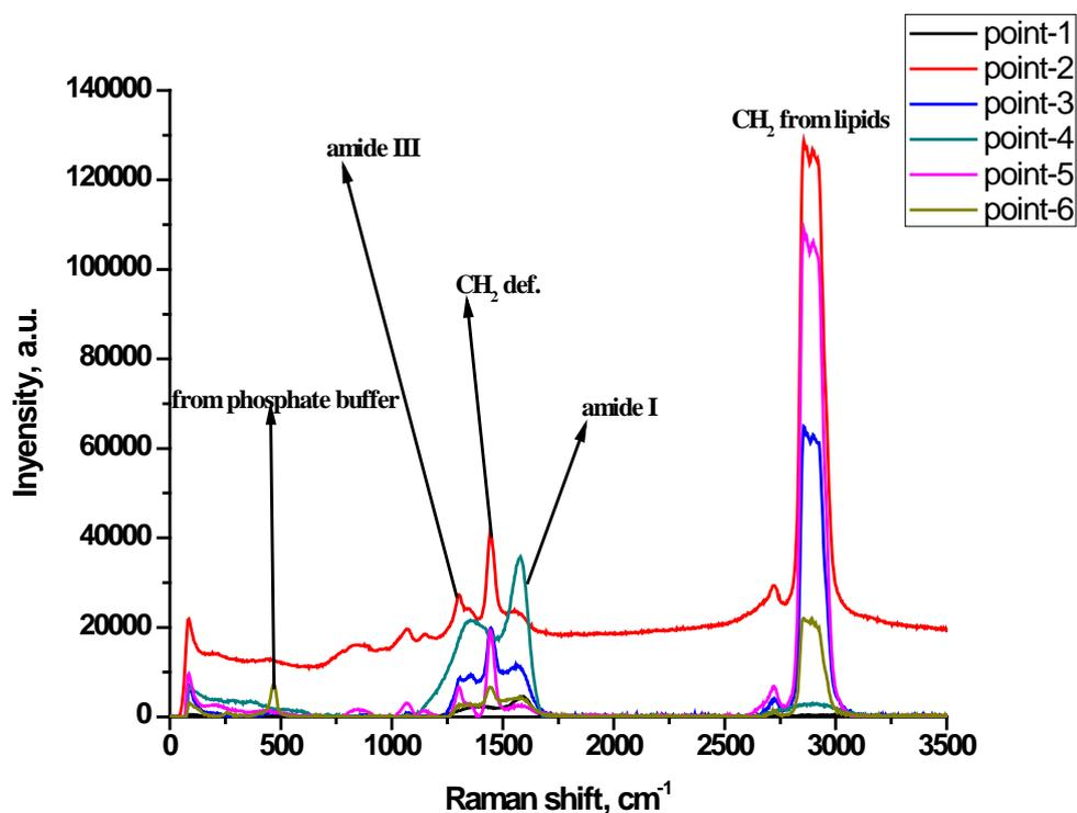
Fig (11): Raman spectrum of SRB biofilm after 12<sup>th</sup> days (steal substrate)
