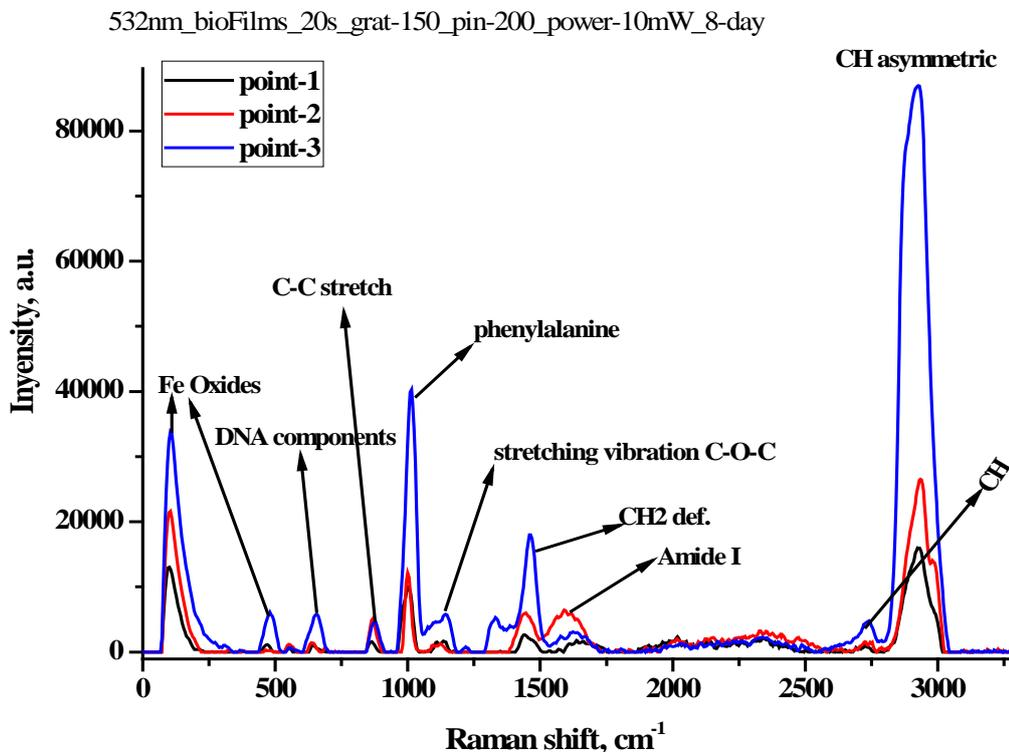
Fig (9): Raman spectrum of SRB biofilm after 8<sup>th</sup> days (scratch the surface of the steal)
