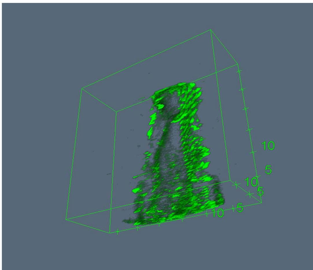
**Fig (15): CARS imaging of SRB biofilm after three days (steel substrate)**
