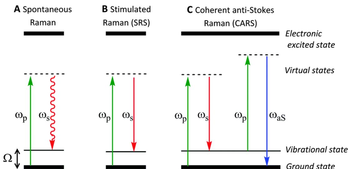
**Fig (2) Energy diagram of (A) spontaneous raman, (B) SRS, and (C) CARS.**
