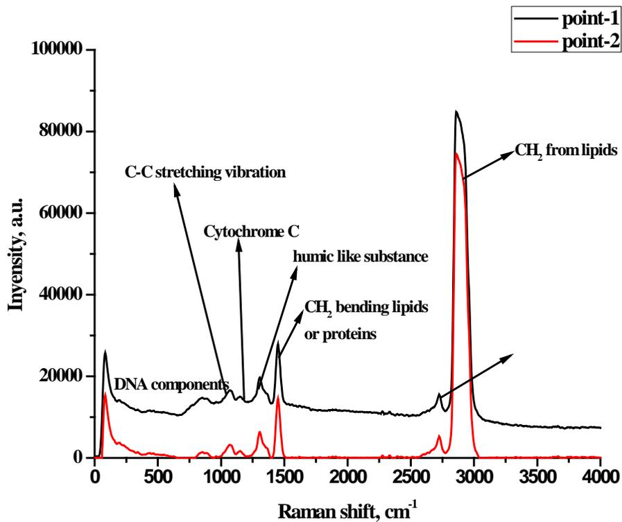
Fig (8): Raman spectrum of SRB biofilm after 7<sup>th</sup> days (scratch the surface of the steal)
