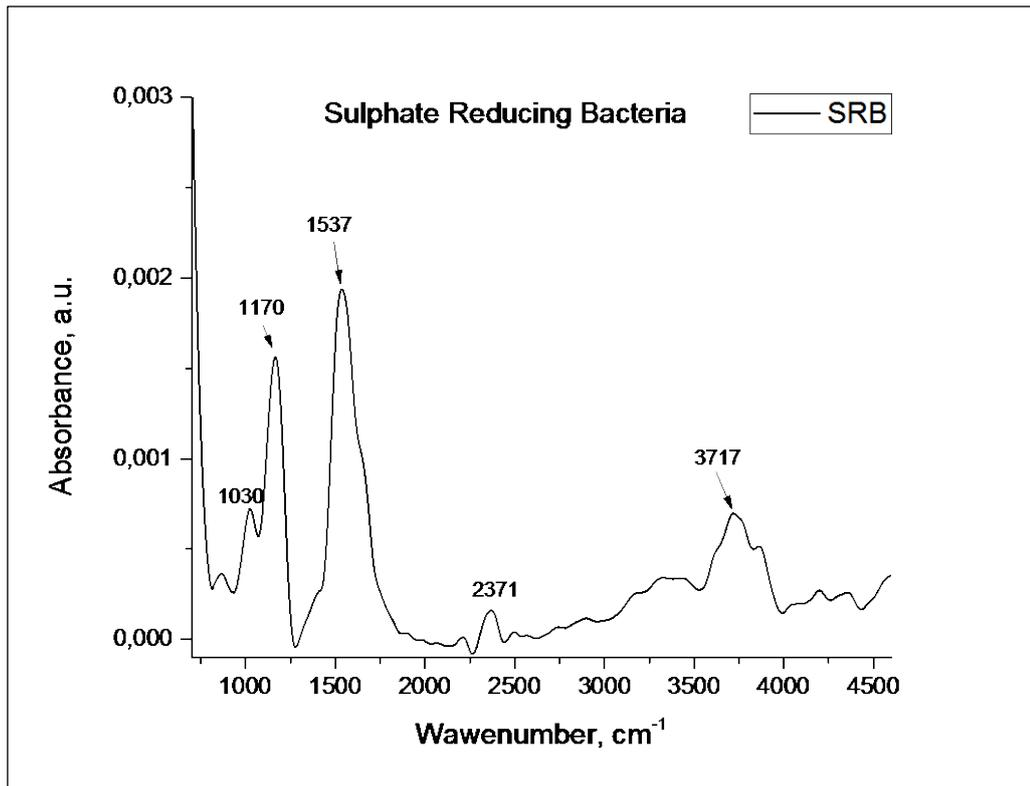
**Fig (15): FT-IR of SRB biofilm (steal substrate)**
