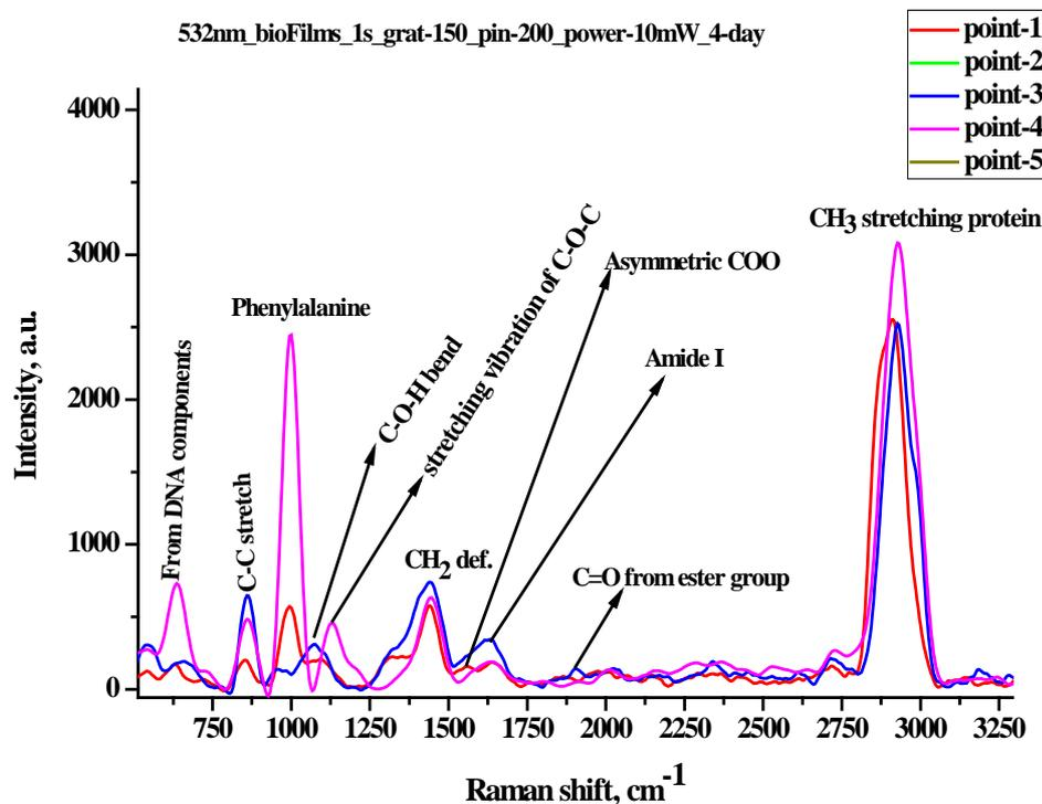
Fig (7): Raman spectrum of SRB biofilm after 4<sup>th</sup> days (scratch the surface of the steel)
