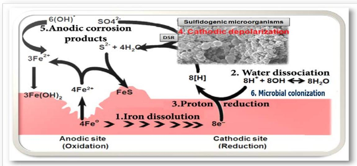
**Fig (5): Corrosion formation.**
