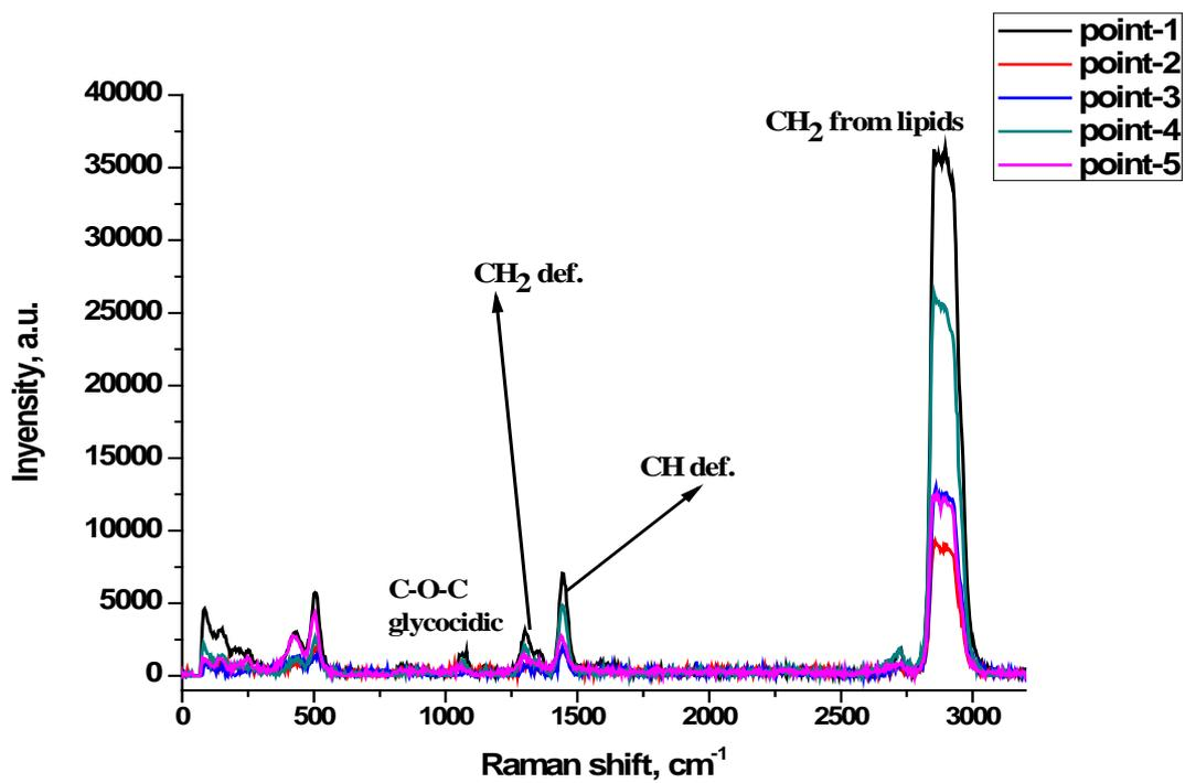
**Fig (14): Raman spectrum of SRB biofilm after 25<sup>th</sup> days (steel substrate)**
