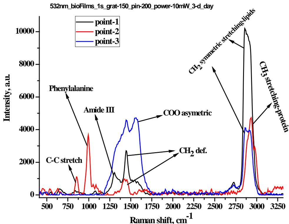
Fig (6): Raman spectrum of SRB biofilm after 3<sup>rd</sup> days (scratch the surface of the steel)
