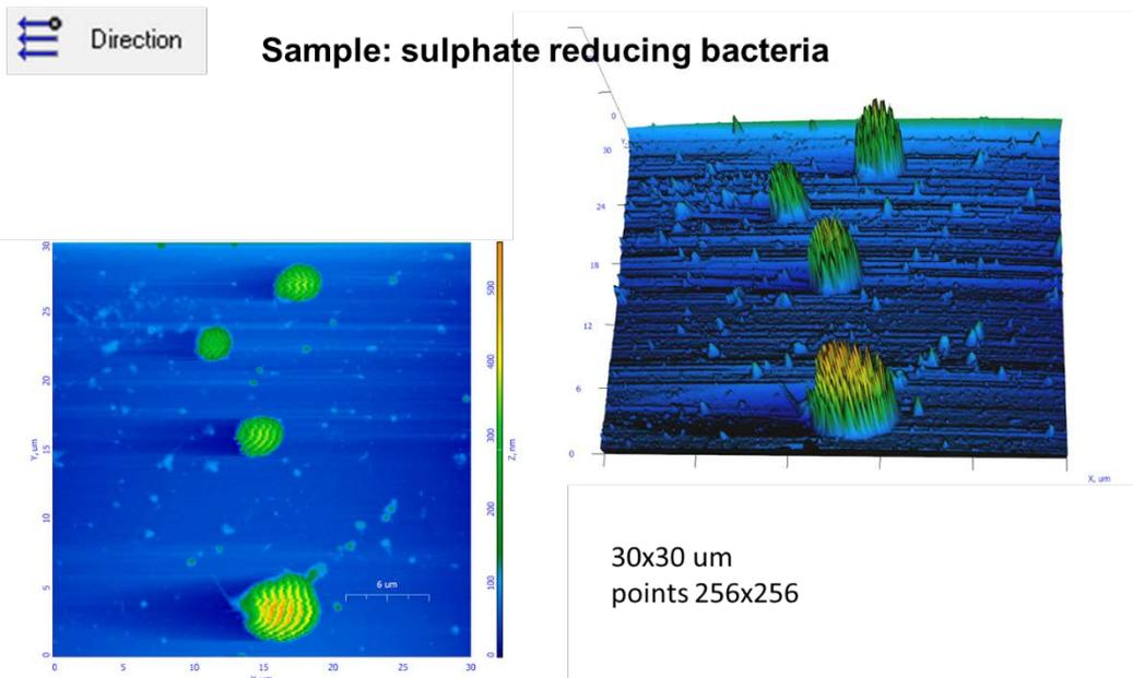
**Fig (16): Atomic force microscope imaging of SRB biofilm after 7<sup>th</sup> days (steal substrate)**
