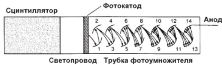
**Fig. 4.** *The typical location of components in a scintillation detector.*
