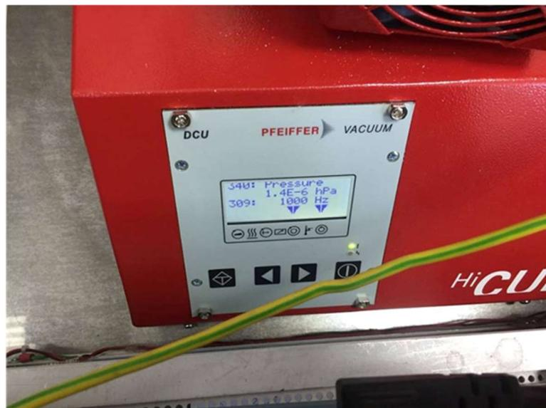
Figure 11. Low pressure which mean good level of vacuum.
