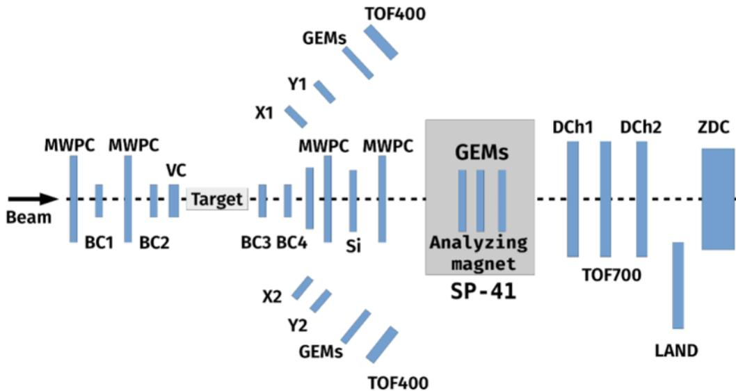
Figure 1: The scheme of the SRC facility
