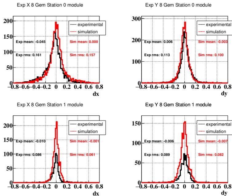
Figure 6: Residuals for the experiment and simulation data. Station 8
