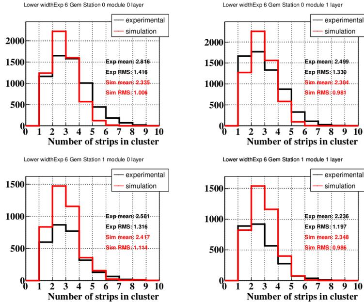
Figure 7: The cluster width in the experiment an simulation
