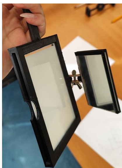
Figure 8. Mirror system used to direct the emitted light towards the camera.
