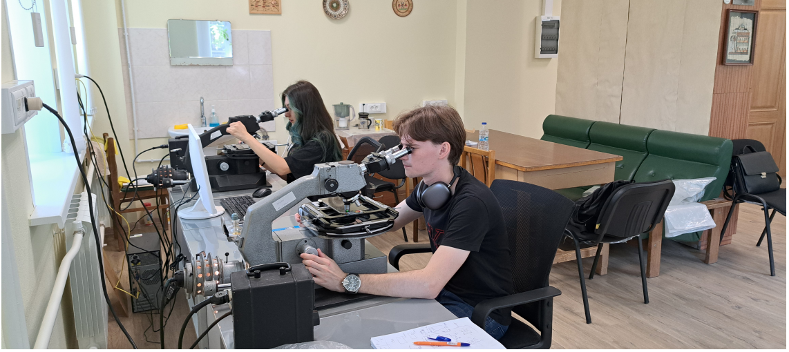
Figure 4: Beam profile measurement using the MBI-9 microscope
