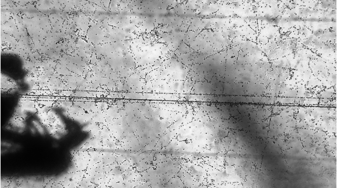
Figure 8: The macro-photograph of tracks, acquired using a motorized Olympus BX63 microscope, reveals intersections between b - and g -particle trajectories. This configuration creates significant risk of misidentifying white star events, potentially generating false fragment + \alpha particle events.
