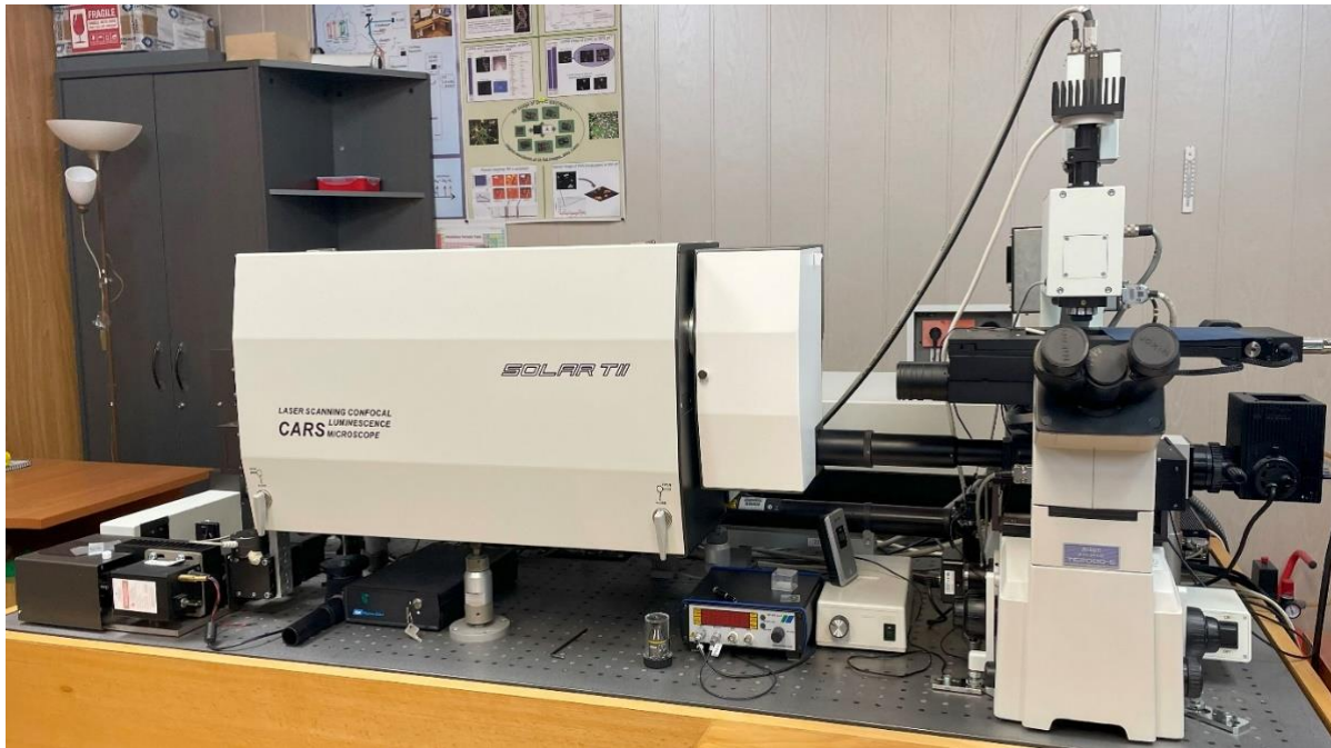
Figure 1. General view on the multifunctional 3D Scanning Laser Microscope – “Confotec CARS”.
