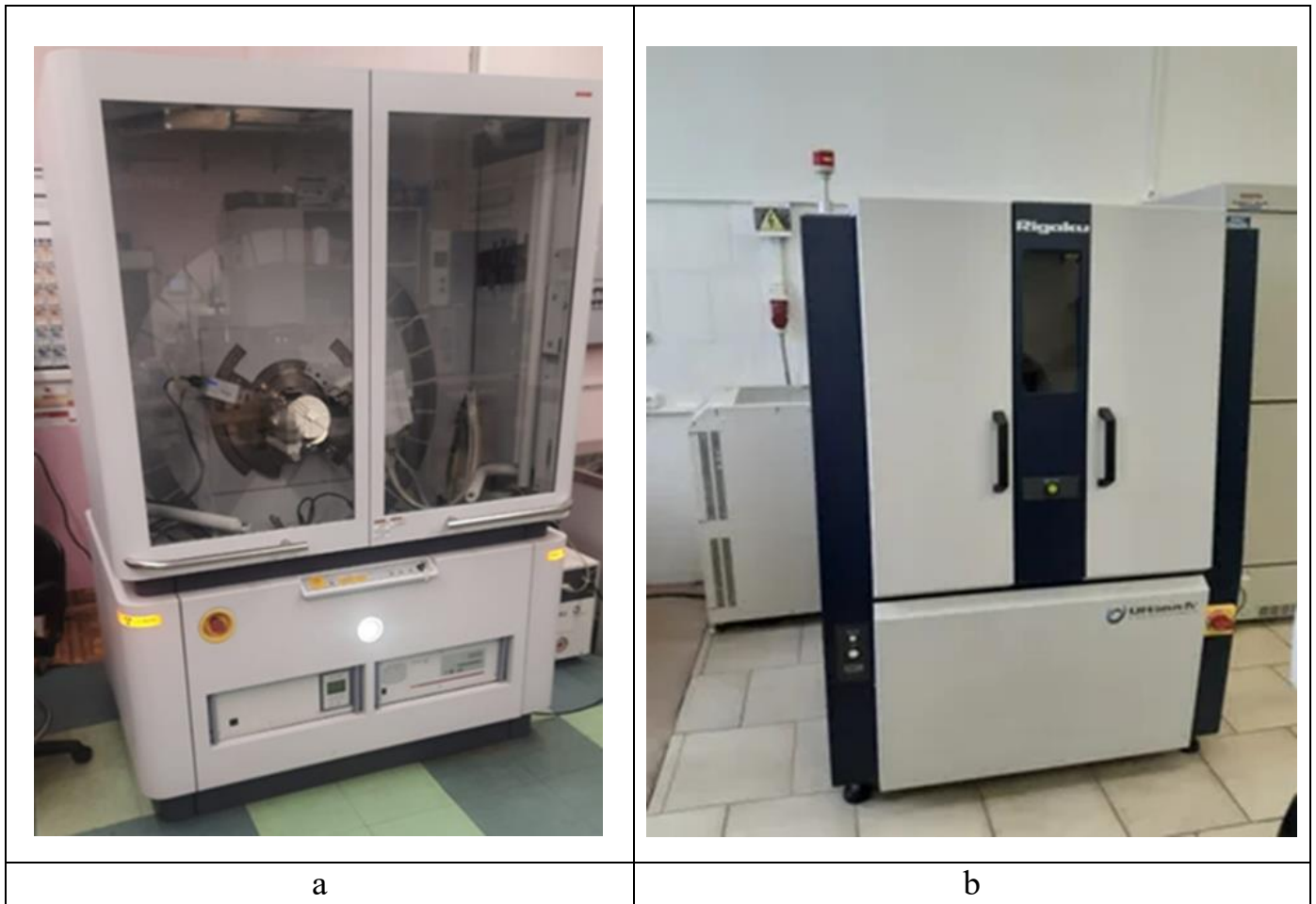
Fig.6. X-ray diffractometers Panalytical (a) and Rigaku Ultima IV (b).
