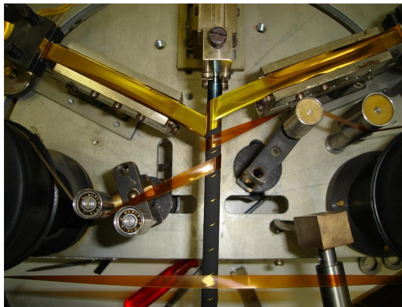
Figure 4. Overall view of the machine used for the production of thin-film polymer tubes.
