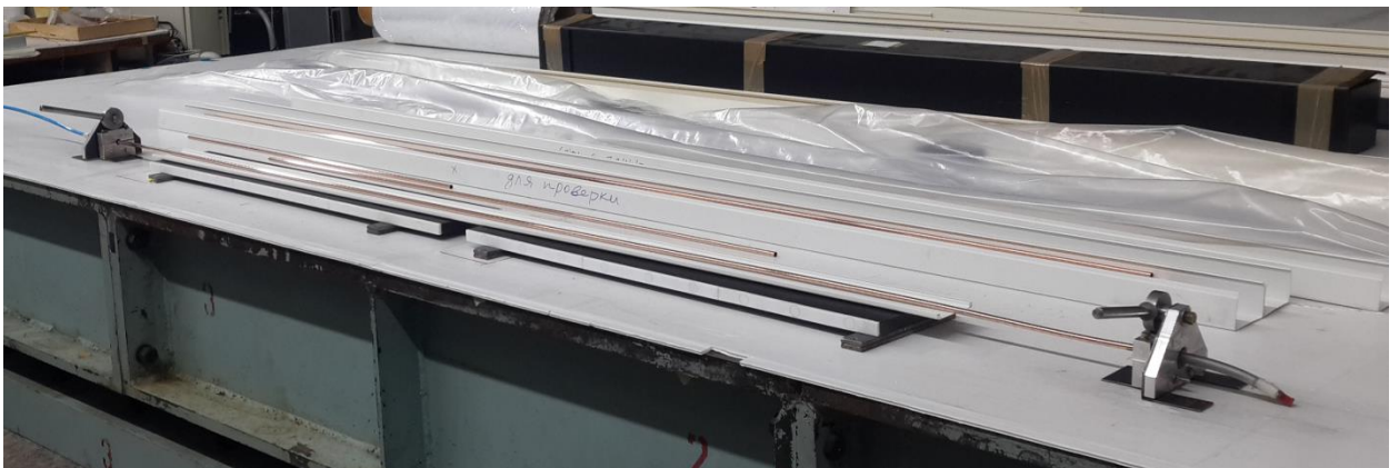
Figure 6. Overall view of the assembly for testing the leak tightness of straw tubes.
