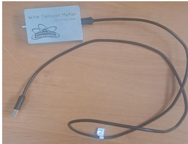
Fig. 6. Device for measuring tension with a USB cable for connecting to a computer.
