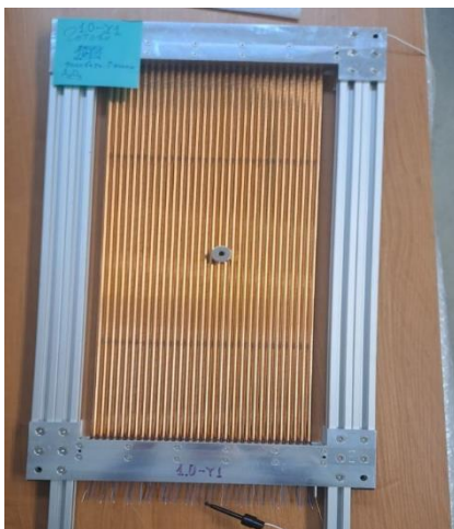
Fig. 4. Preliminary tension measurement with a magnet.
