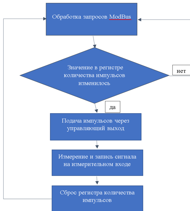
Figure 8. Block diagram of STM32 software operation.
