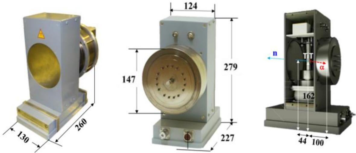
**Fig.3** ING-27 dimensions (mm) and the direction of irradiation of DT-reaction fragments.
