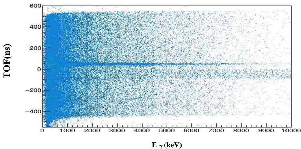
**Fig. 8** Two Dimensions histogram of gamma coincidence with alpha. This figure 6 depicts the raw data spectrum from the MCA (multichannel analyser). We obtained this spectrum data from HPGe utilizing the data acquisition system.
