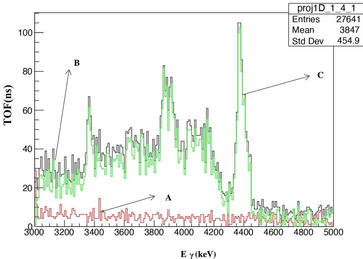
**Fig.9**  $\gamma$ -energy spectrum measured with HPGe detectors for  $^{12}\text{C}$ . Green line for Subtracted data(C) and black one is raw data (B) and red one is the Background data(A).
