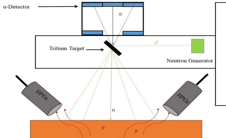
**Fig.1** Layout of tagged neutron method [4].
