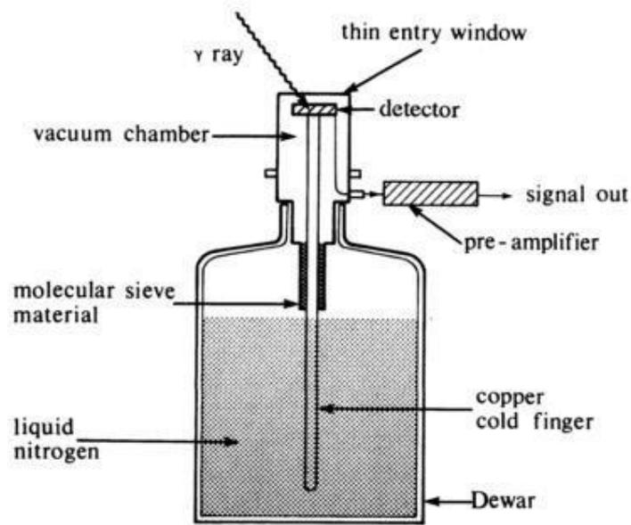
**Fig.5** Fundamental layout of HPGe Detector
