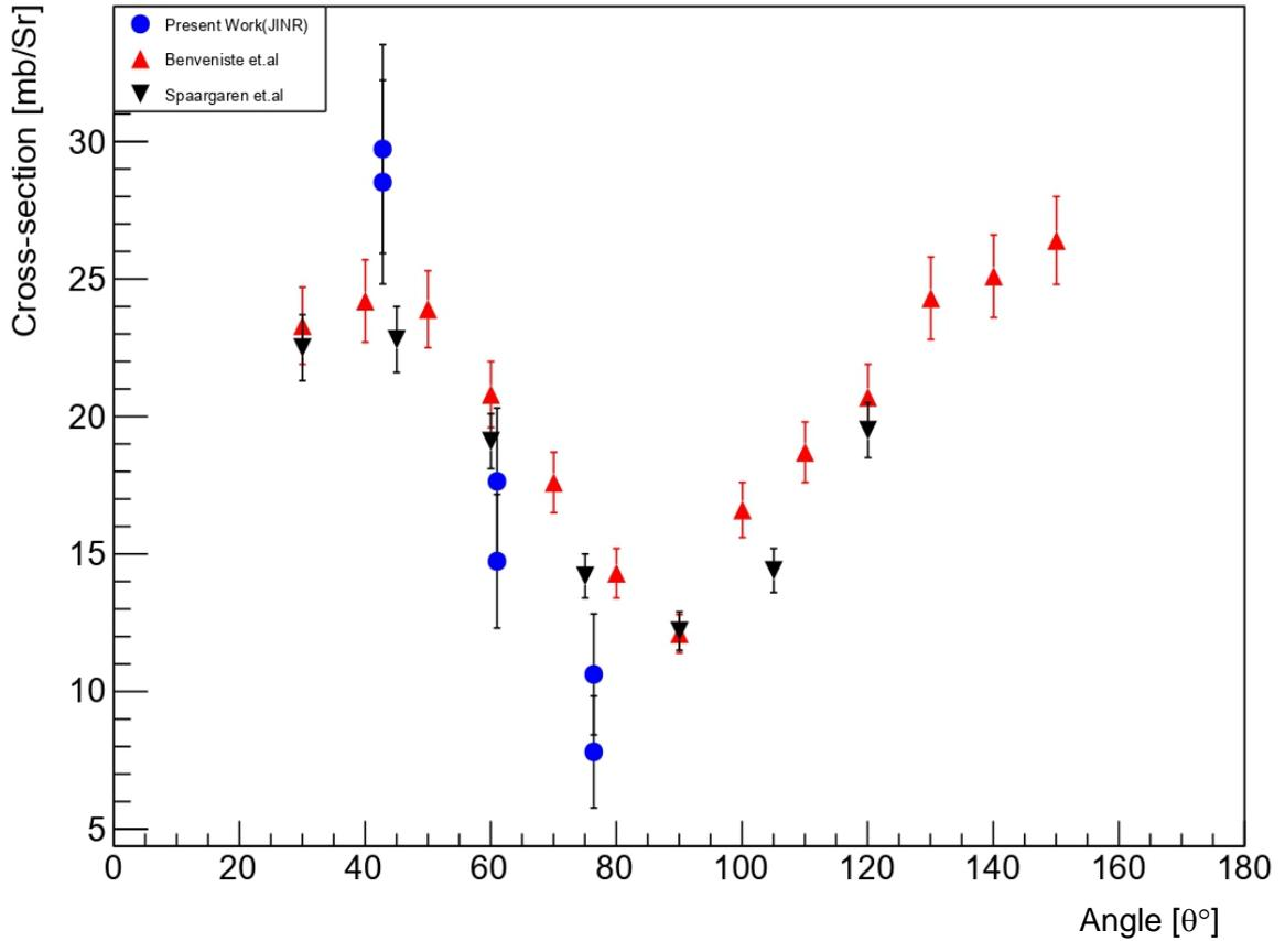
**Fig.12** Comparison of the experimentally measured angular distribution for  $^{12}\text{C}$  ( $n, n\gamma$ ) with the existing experimental data.
