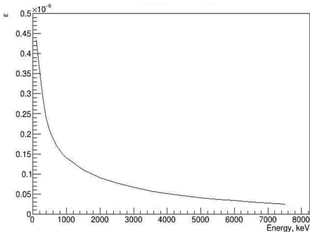
**Fig.11** Estimated efficiency from the Monte-Carlo method in GEANT4
