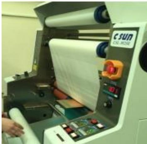
*Figure 3. Lamination of a prototype at JINR DLNP*
