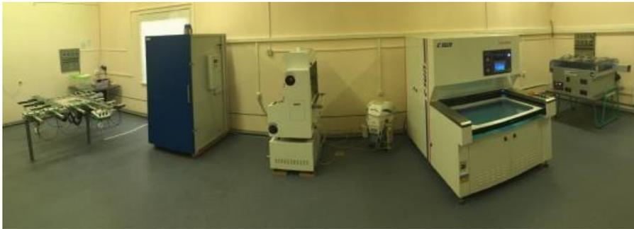
*Figure 2. Fabrication chain at JINR DLNP. From left stretching machine, oven, laminator, UV insulator, etching machine*
