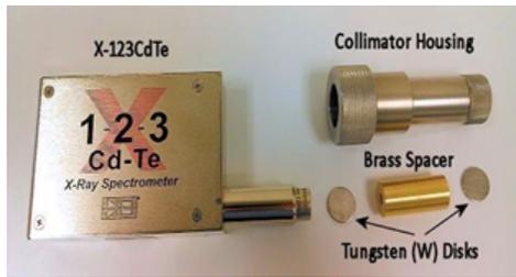
**Fig. 3:** Shows X-123 CdTe detector.
