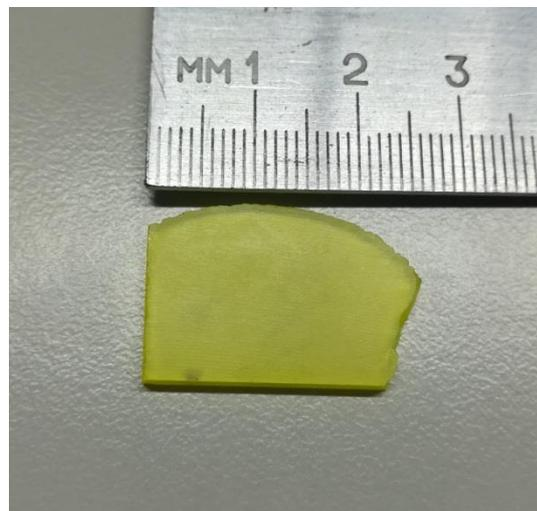
Fig. 1a. Experimental sample of single crystal  $\text{Gd}_3\text{Ga}_5\text{O}_{12}$ : Al. The sample was provided by Fomos-MaterialisGroupe
