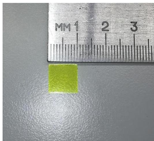
Fig. 1a. Experimental sample of single crystal  $\text{Gd}_3\text{Ga}_5\text{O}_{12}$ : Ce. The sample was provided by Fomos-MaterialisGroupe
