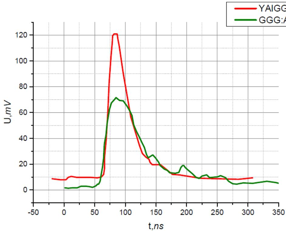
Fig. 12. The graph comparing the responses from the pulses of GGG: AL and YGGG: Ce
