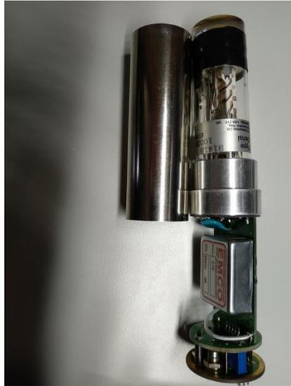
Fig. 5. The tube of  $\mu$ metal near the photoelectric multiplier device
