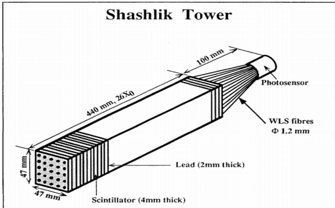
Figure A. The example mechanical design of a CMS Shashlik calorimeter prototype tower equipped with 25 aluminized WLS fibres. Side view.
