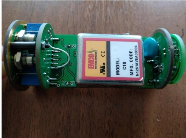
Fig. 4a. the module of electronic of the photoelectric multiplier ETEnterprises model 9106sb
