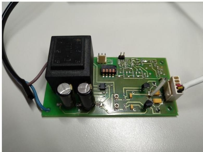
Fig. 4 b. Power supply ETEnterprises model 9106sb
