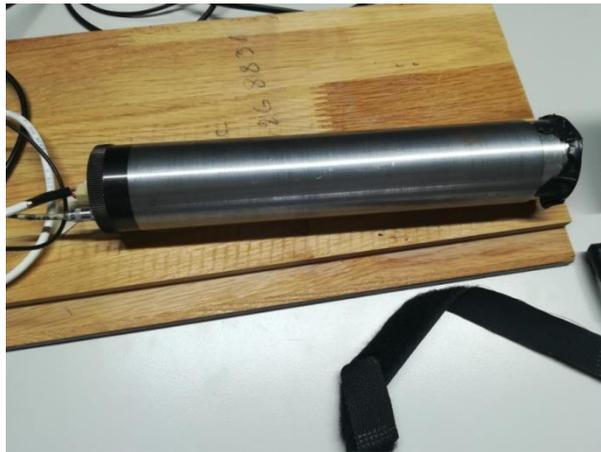
Fig. 2a. The photo of the photoelectronic multiplier used in the experiment. Side view.
