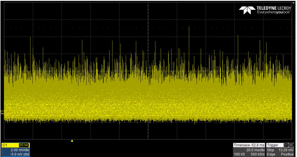
Fig. 11. The level of the noise path when measuring the pulse on an oscilloscope was not more than  $\pm 4\text{mV}$
