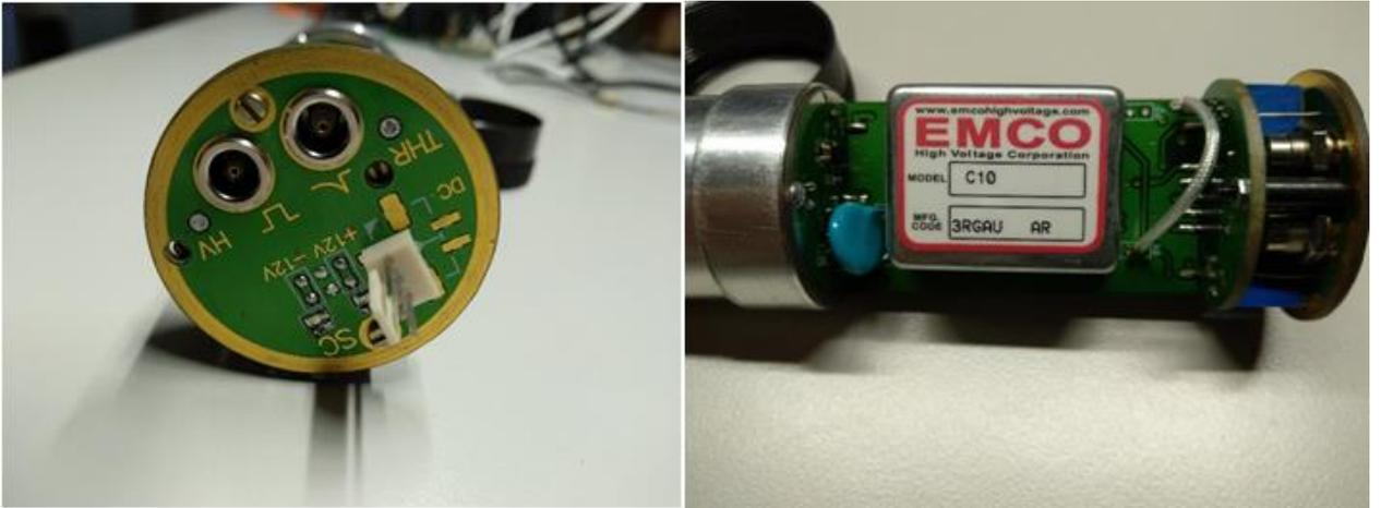
Fig. 2c. Photo of the photomultiplier assembly with amplifier and high-voltage converter EMCO.
