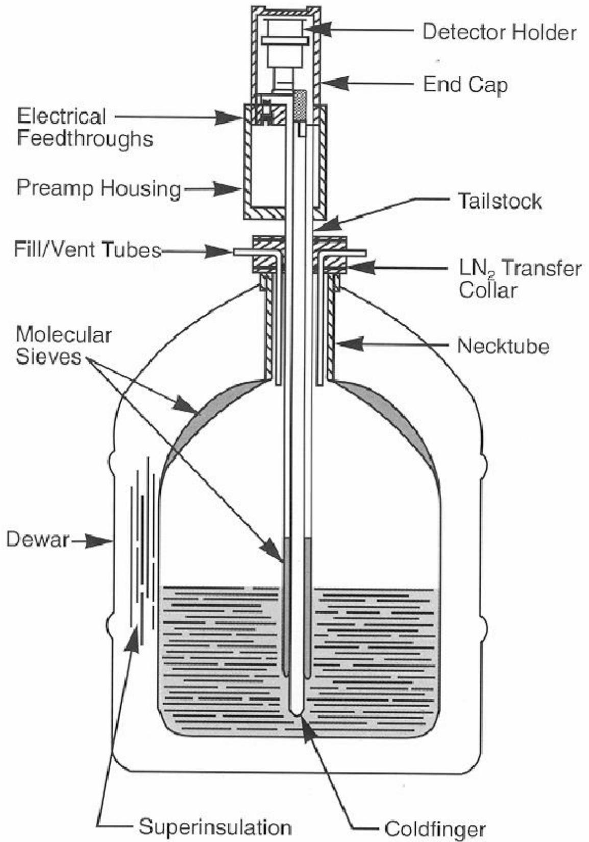
**Fig. 1. HPGe detector in a cryostat**
