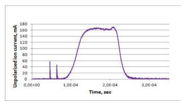
Figure 21. Unpolarized ion current (D+) downstream the analyzing magnet
