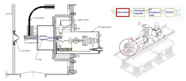
Figure 12. Schematic layout of RF dissociator with specification of its location
