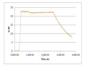
Figure 19. Accelerating voltage pulse: 22kV, 300 µs
