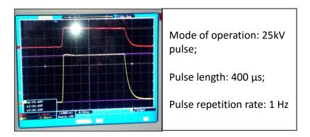
Figure 15. Hydrogen plasma source HV pulse generator
