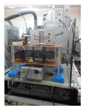
Figure 17. Power supplies for the plasma source
