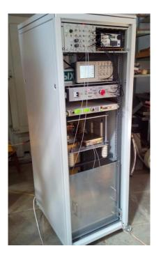
Figure 16. High-voltage pulse generator of the arc plasma source
