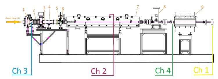
Figure 5. Schematic layout of the experiment: 1 – Electrostatic lenses (E1 and E2); 2 – Electrostatic pre-accelerator; 3 – Magnetic lens L1; 4 – Corrector; 5 – Magnetic lens L2; 6 – Faraday cup; 7 – RFQ module; 8 – Buncher; 9 – Magnetic analyzer;
