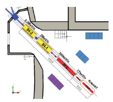
Figure 3. HILAC and its components
