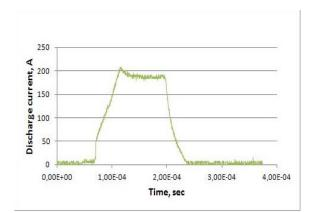
Figure 20. Discharge current pulse of the plasma source, 200 A peak, 100 µs
