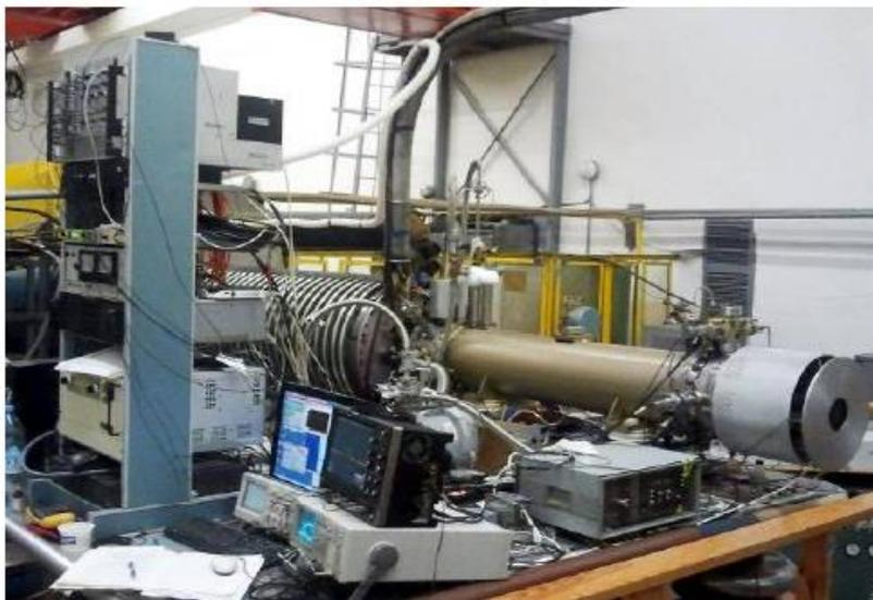
Figure 3.2 Krion-6T at high-voltage platform of LU-20 fore-injector. The Nuclotron Run #50.
