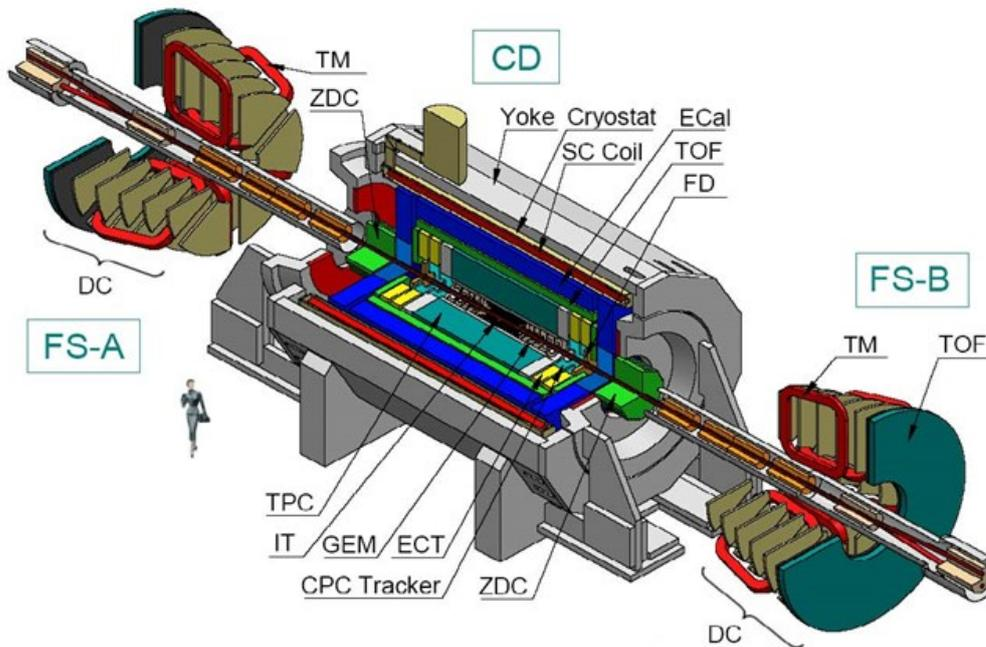
Figure 2. MPD (Multi Purpose Detector)
