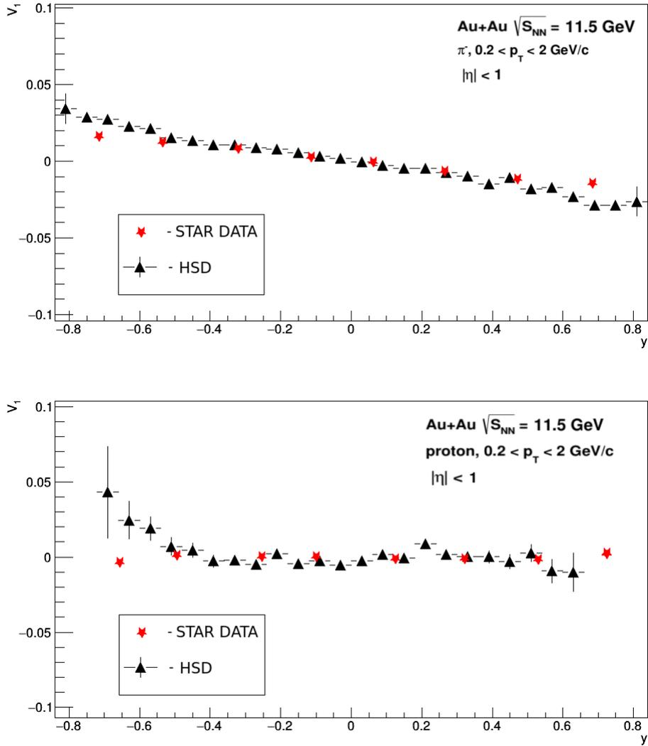
Figure 4. Directed flow  $v_1$  for protons and  $\pi$ -mesons Au+Au collision at collision energies  $\sqrt{S_{NN}} = 11$  GeV derived from the HSD. The experimental data are from the STAR collaboration. The following cuts were applied:  $|\eta| \leq 1$ , centrality is 10-40%, the experimental acceptance  $0.2 \leq P_T \leq 2$  GeV/c is taken into account for all hadrons.
