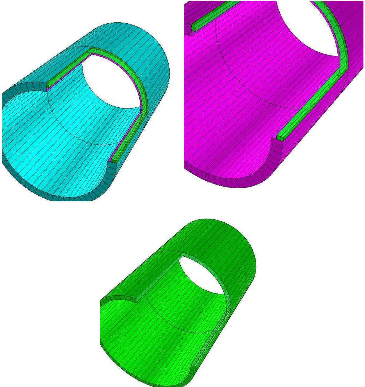
Fig. 8 Cryostat assembly. The steel walls of the cryostat (blue), the volume of the vacuum (lilac), the solenoid (green)
