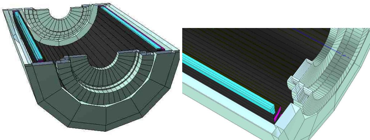
Fig. 2 Structure of the magnet and cryostat in the section in the original geometry. Clearly visible are all the segments of which the magnet and the cryostat consist.
