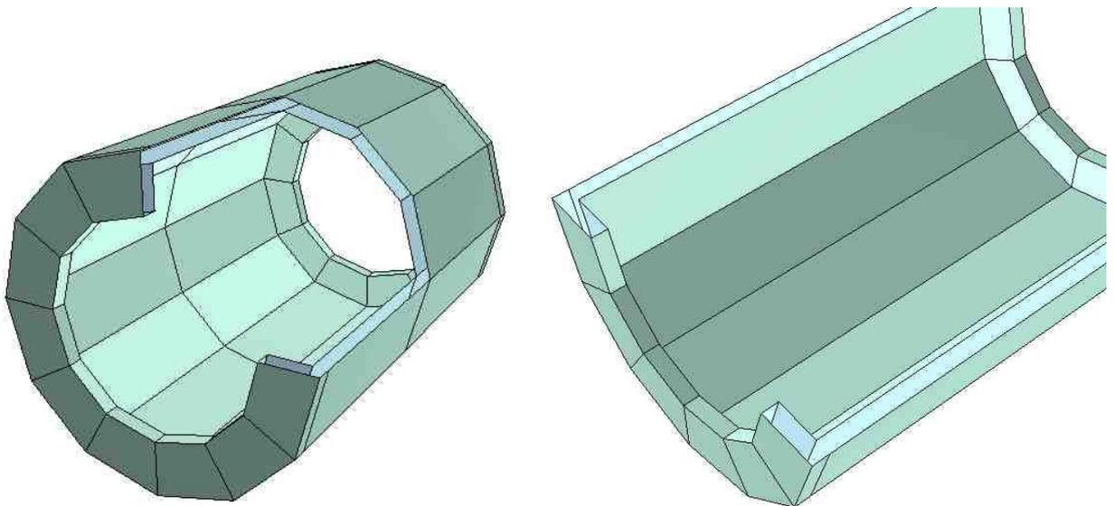
Fig. 11 Barrel magnet and part of the end volumes after optimization
