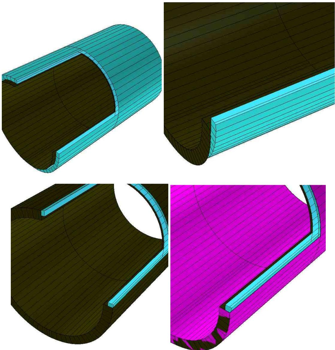
Fig. 7 Inside the cryostat the cryostat solenoid (blue), the cryostat walls of steel (black), the vacuum between the solenoid and the steel walls (lilac)
