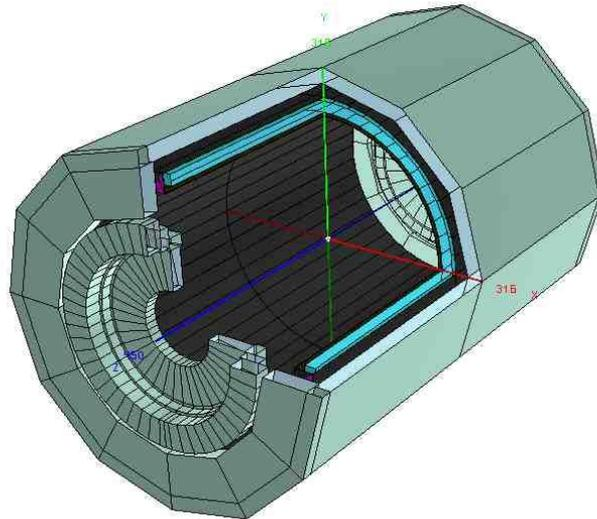
Fig. 3 Magnet of the detector MPD.
