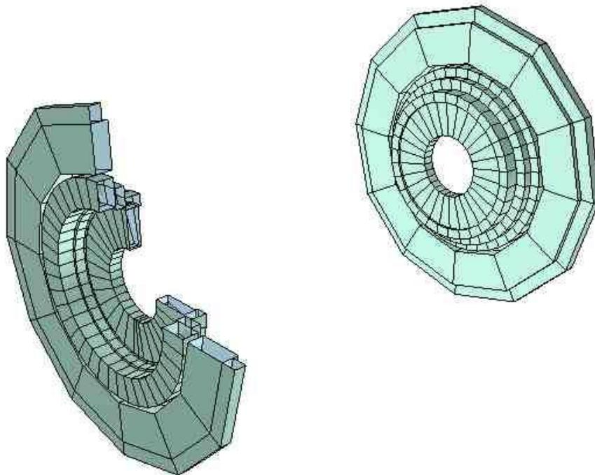
Fig. 4 Volumes constituting the end parts of the magnet.
