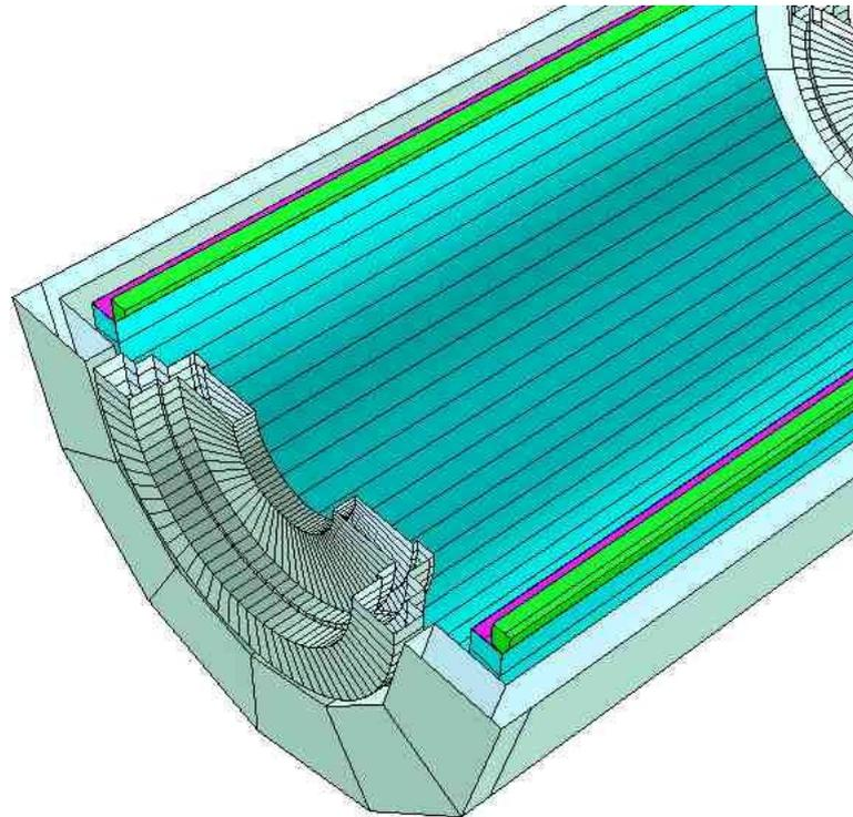
Fig. 12 Magnet and cryostat after transfer to new geometry and optimization
