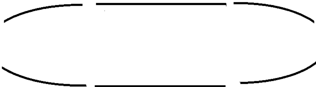
Figure 4.3: Three segment symmetrical parabolic neutron guide system
