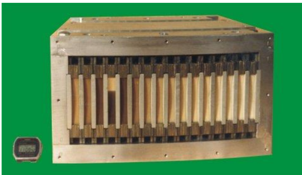
Figure 4.8: Focusing collimator used in neutron experiments
