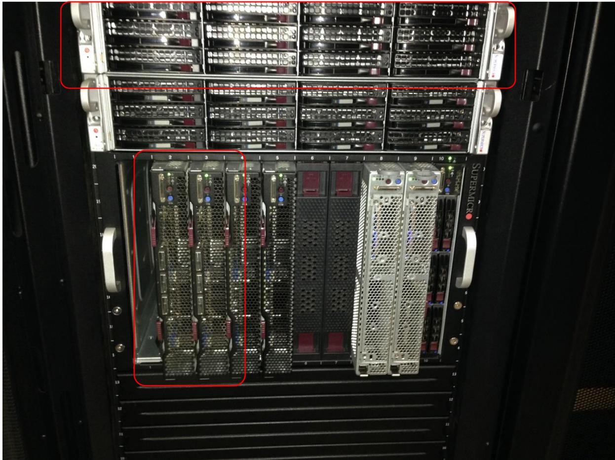
*Figure 1: part of Hybrilit cluster, parts provided for experimentation selected in red. A server node and two blades.*
