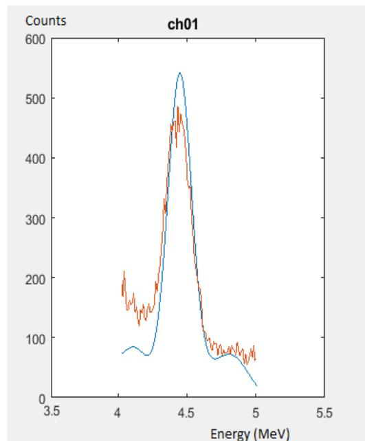
Figure 6.b. Validation of MCNP results on experimental results for detector 01.
