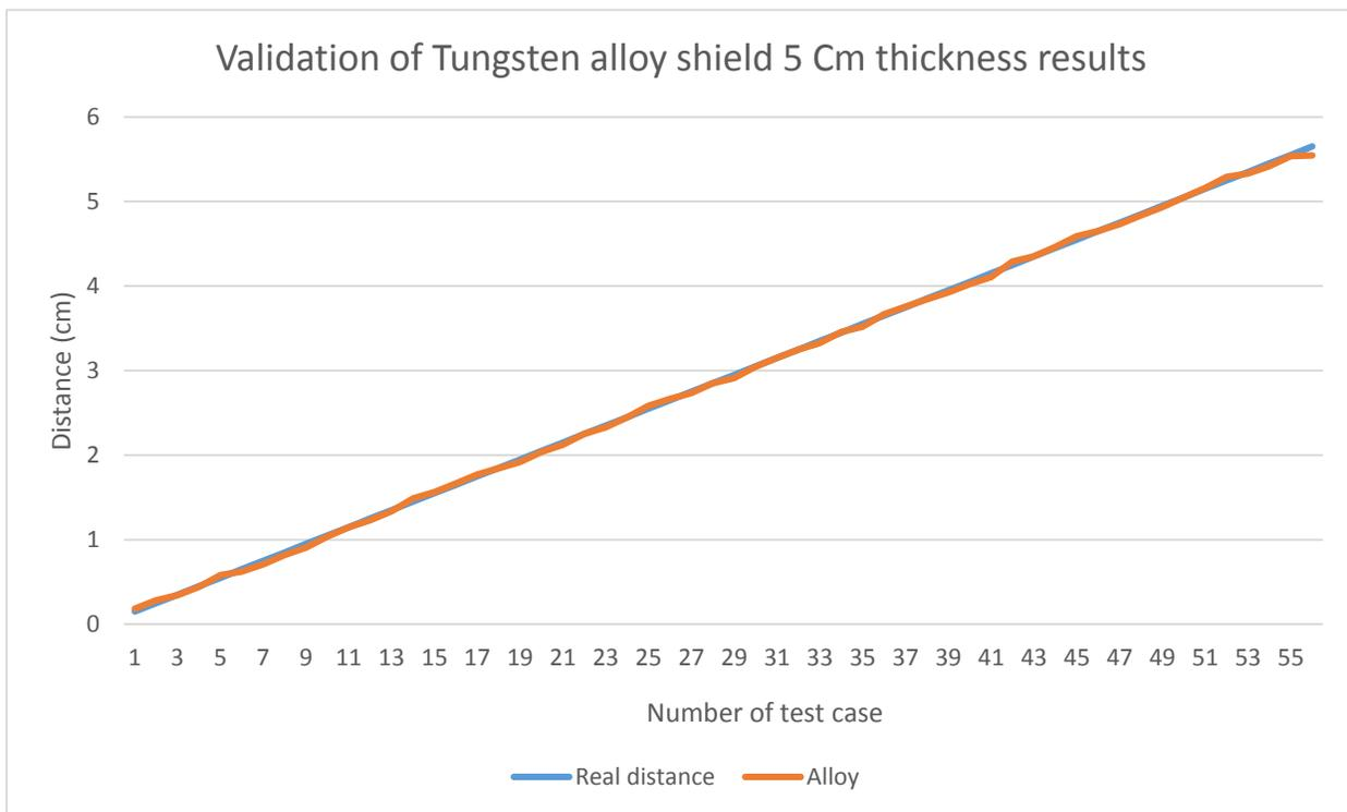
Figure 11.f. Validation of Neural net fitting algorithm on MCNP results based on 56 test cases for Tungsten alloy shield with thickness = 5 cm.
