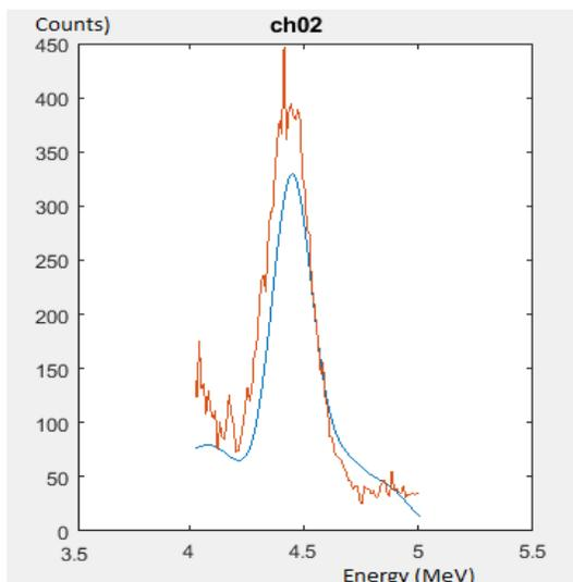
Figure 6.c. Validation of MCNP results on experimental results for detector 02.
