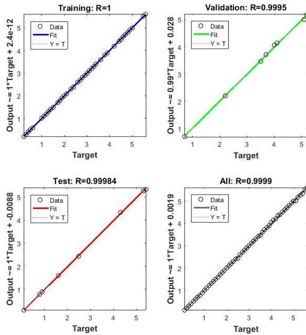
Figure 10.e. Predictor Regression of NNF for Tungsten shield with thickness= 5 cm.
