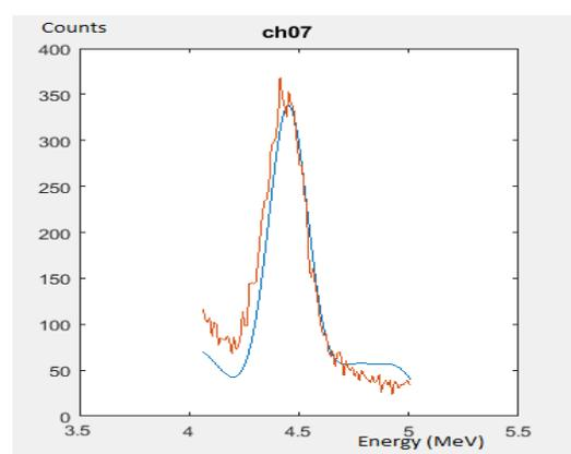
Figure 6.h. Validation of MCNP results on experimental results for detector 07.
