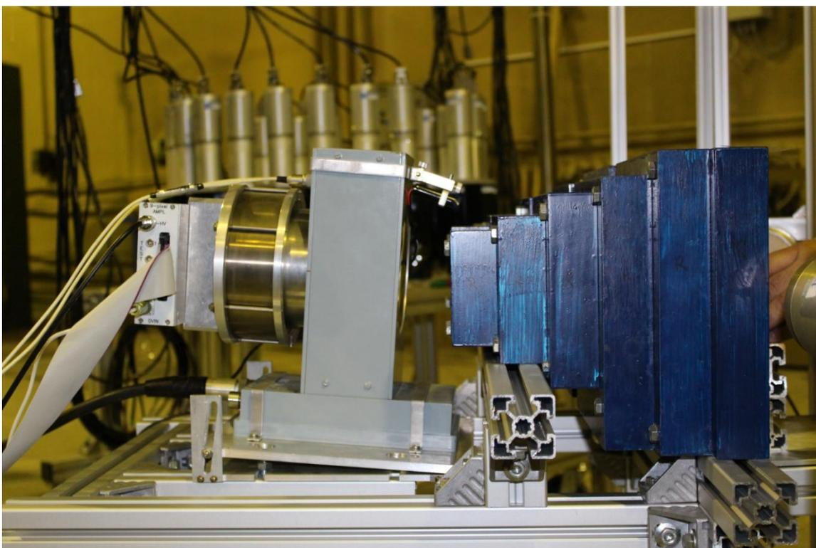
Figure 4. Neutron generator ING-27 and the iron shielding-collimator.
