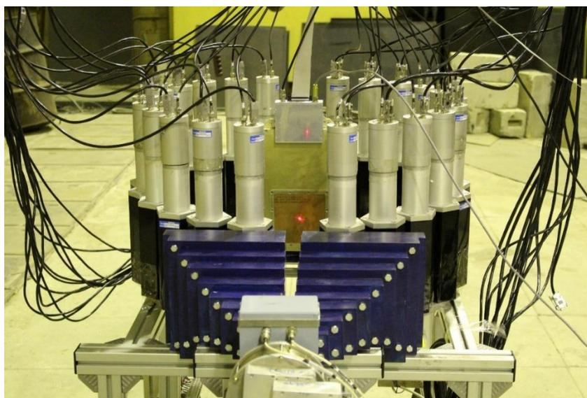
Figure 2. ROMASHKA setup, 22 hexagonal NaI (TI) gamma-ray detectors.
