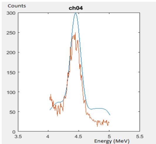
Figure 6.e. Validation of MCNP results on experimental results for detector 04.
