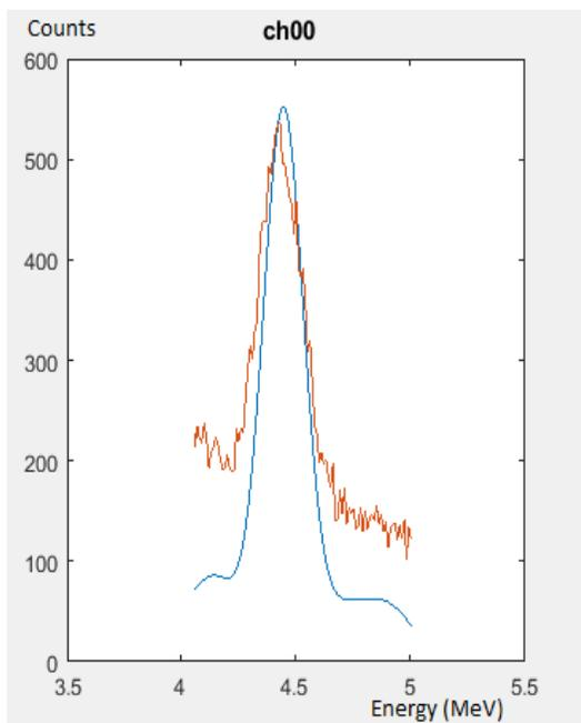
Figure 6.a. Validation of MCNP results on experimental results for detector 00.
