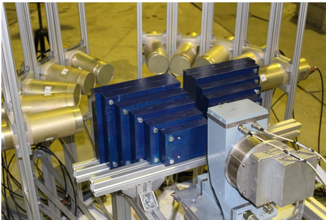
Figure 3. ROMASHA setup, 10 BGO (Bi<sub>4</sub>Ge<sub>3</sub>O<sub>12</sub>) detectors.
