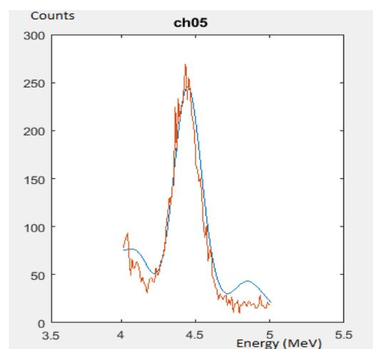
Figure 6.f. Validation of MCNP results on experimental results for detector 05.
