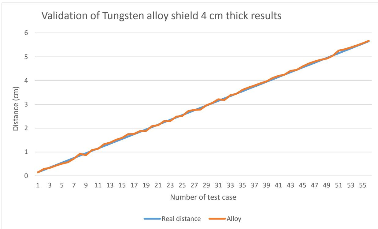
Figure 11.c. Validation of Neural net fitting algorithm on MCNP results based on 56 test cases for Tungsten alloy shield with thickness = 4 cm.
