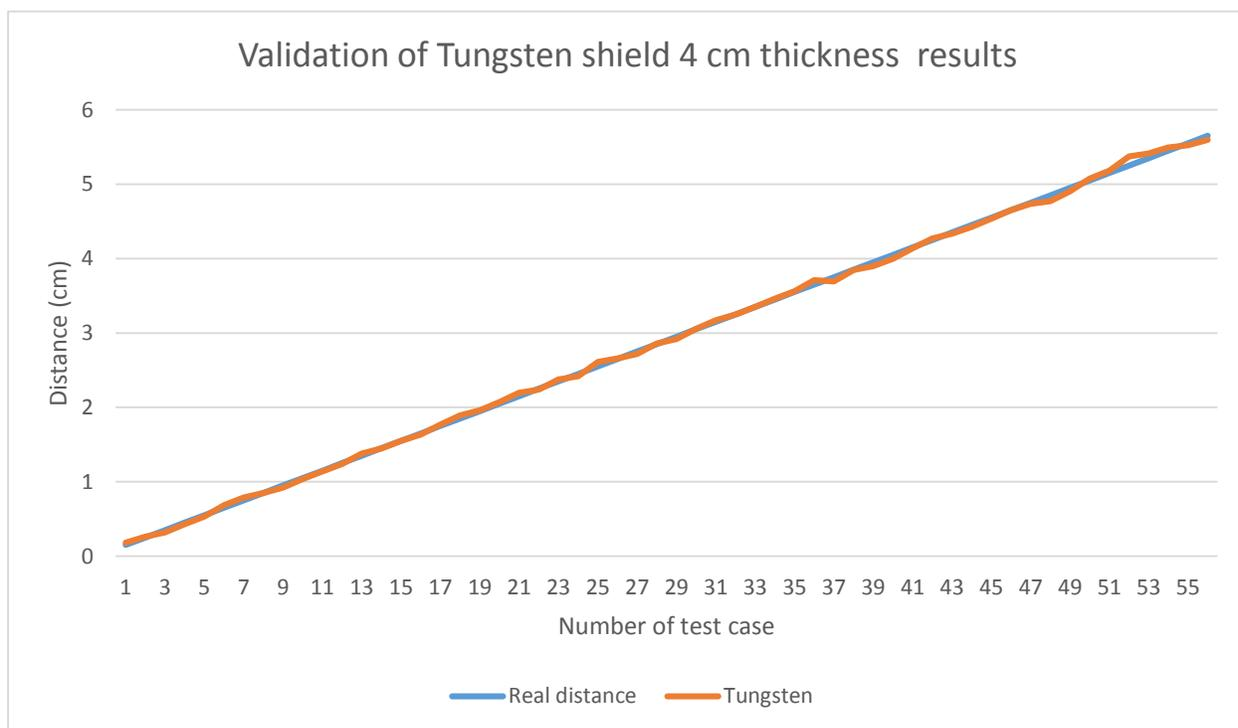
Figure 11.b. Validation of Neural net fitting algorithm on MCNP results based on 56 test cases for Tungsten shield with thickness = 4 cm.
