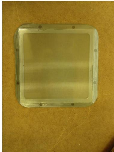
Figure 5: Mesh glued on its frame for a "floating mesh" prototype
