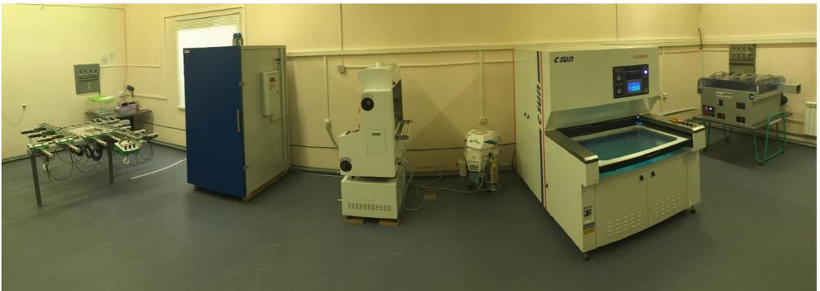
Figure 3: Fabrication chain at JINR DLNP. From left stretching machine, oven, laminator, UV insulator, etching machine
