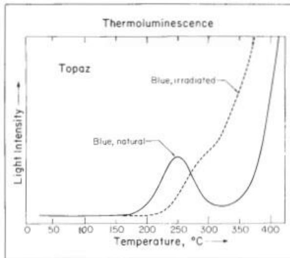
*Fig. 12. Comparison of the thermoluminescence curves of natural and irradiated blue topaz. Only the hightemperature behavior is useful for distinction. The broad emission at 250°C is not present in all natural samples.*
