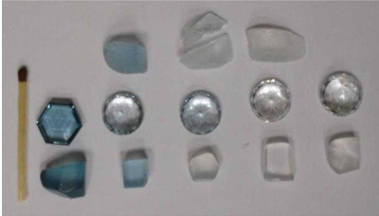
Fig. 18. Topaz samples after the heat treatment (from left to right).
