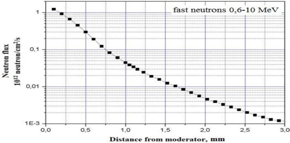
Fig. 7. Dependence of the neutron flux from distance from the moderator for fast neutrons
