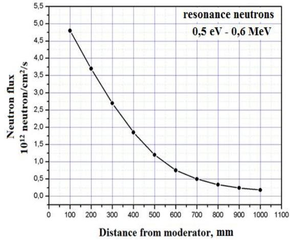
Fig. 9. Dependence of the neutron flux from the distance from the moderator for resonance neutrons.
