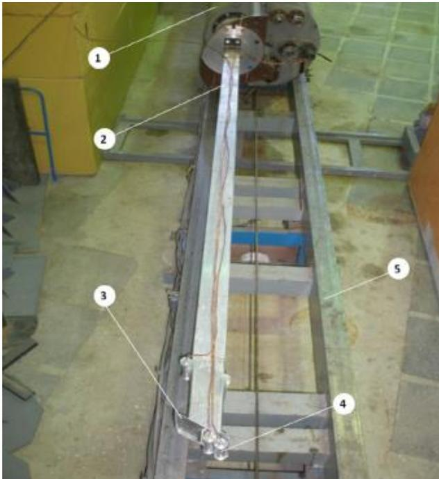
*Fig. 4. The irradiation facility at the channel No. 3 of IBR-2 reactor experimental hall, the view from the external biological shield side: 1 – massive part of the irradiation facility, 2 – transport beam, 3 – metallic container for samples fastening, 4 – samples, 5 – rail way.*
