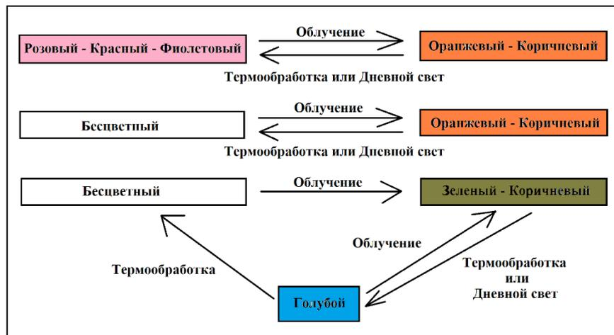
Fig. 17. The color change of topazes at treatment with irradiation and/or annealing (in some cases at exposure of daylight).
