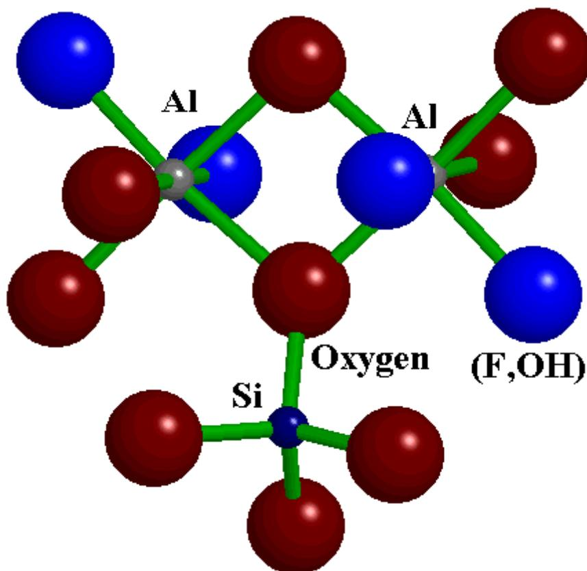
*Fig. 10. The molecular structure of topazes.*
