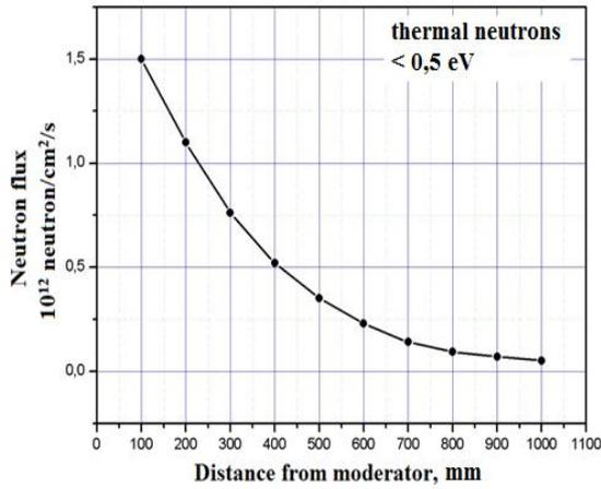
Fig. 8. Dependence of the neutron flux from the distance from the moderator for thermal neutrons.
