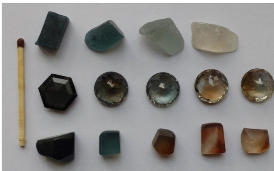
*Fig. 16. The irradiated samples of topazes (from left to right).*
