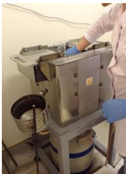
Fig 6 Measurement of 195m Pt sample on HPGe detector
