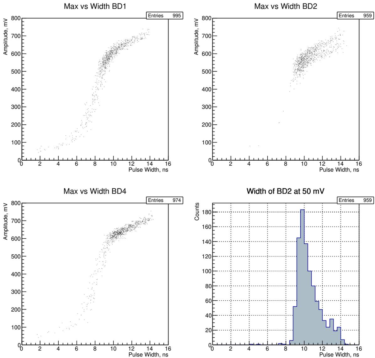
Figure 12: BD Strips: pulse width versus amplitude
