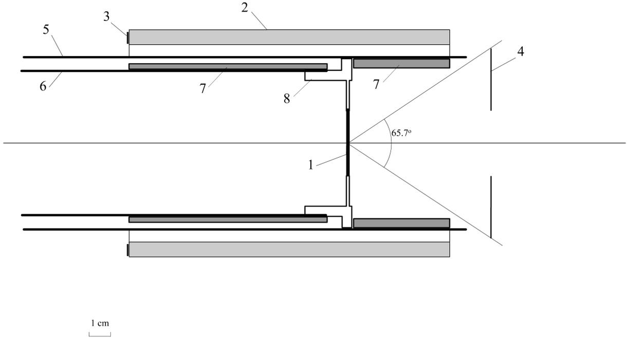
Figure 9: Detailed view of Barrel Detector components. 1 - target, 2 - scintillator strips, 3 - SiPMs.
