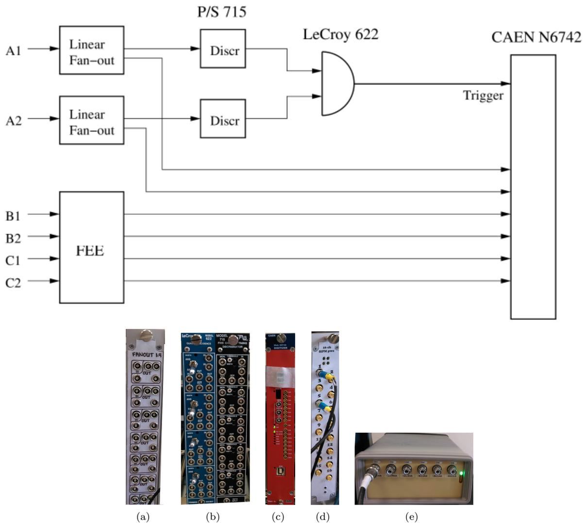
Figure 3: Read-out electronics and components. a) FANOUT system, b) LeCroy 622 and P/S 715, c) CAEN N6742 d) SiPMs power supplies e) PMTs power supplies.
