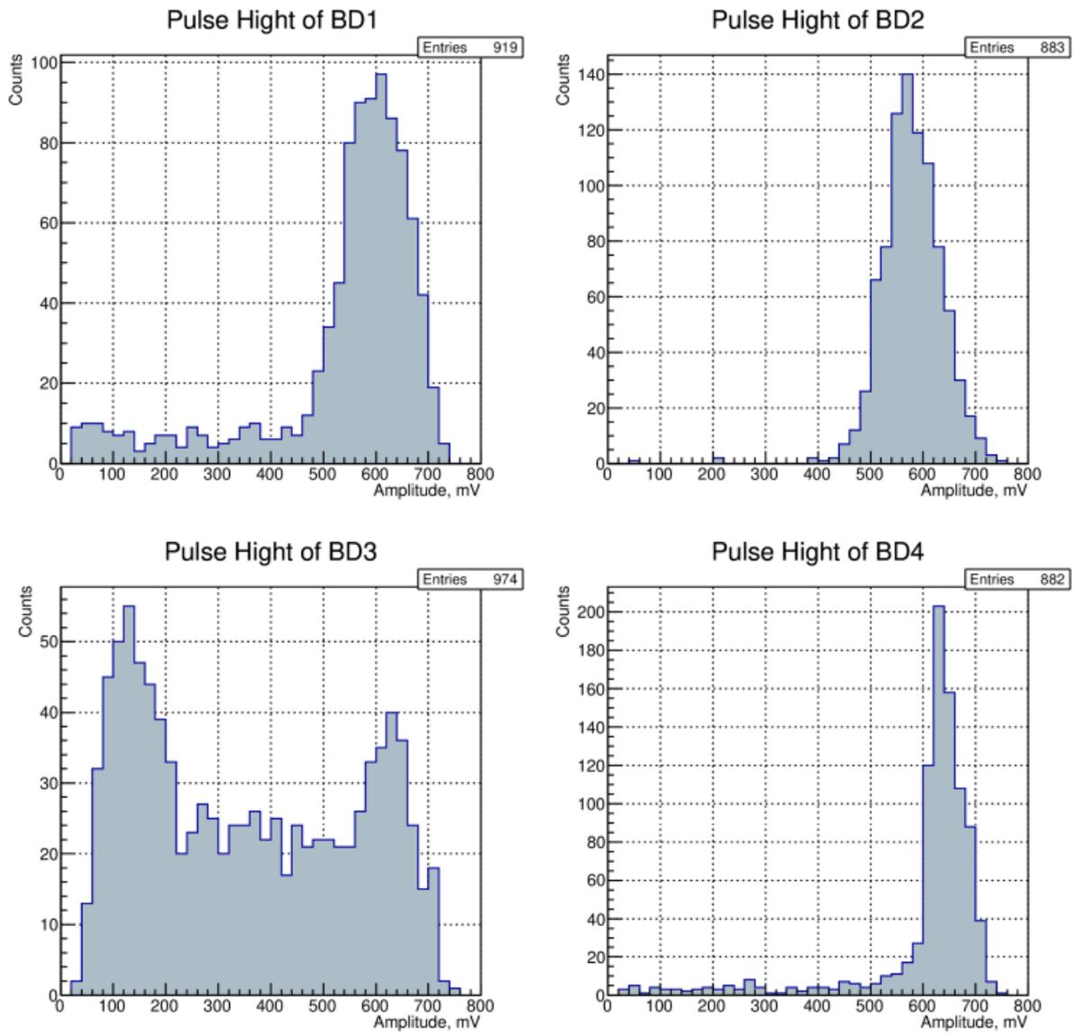
Figure 13: Amplitude distributions of the signals from BD strips.
