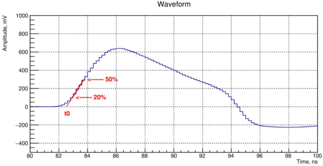
Figure 16: Determination of the signal arrival time.
