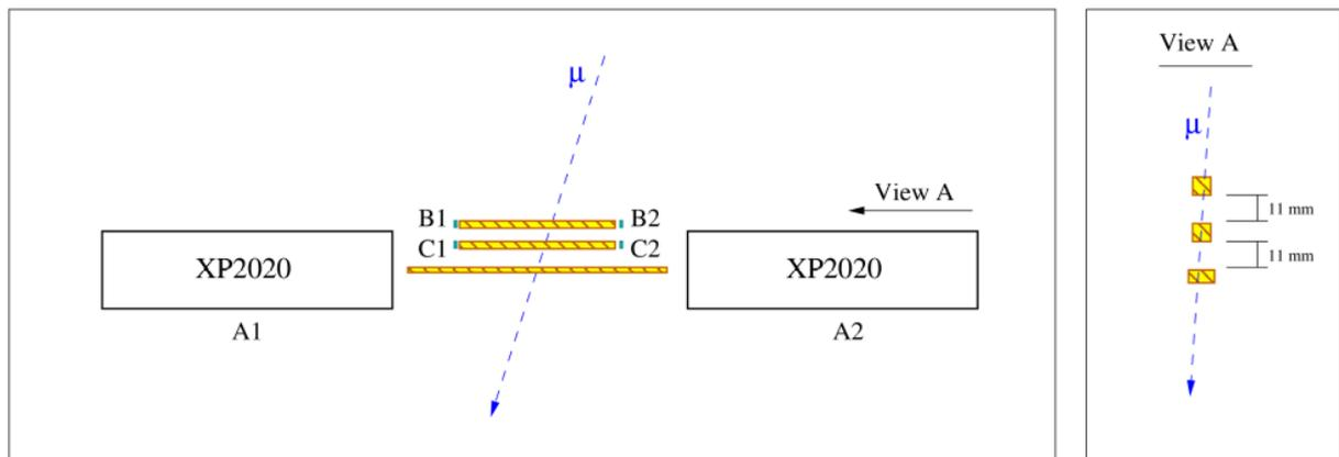
Figure 14: Placement of counters in the time resolution test.
