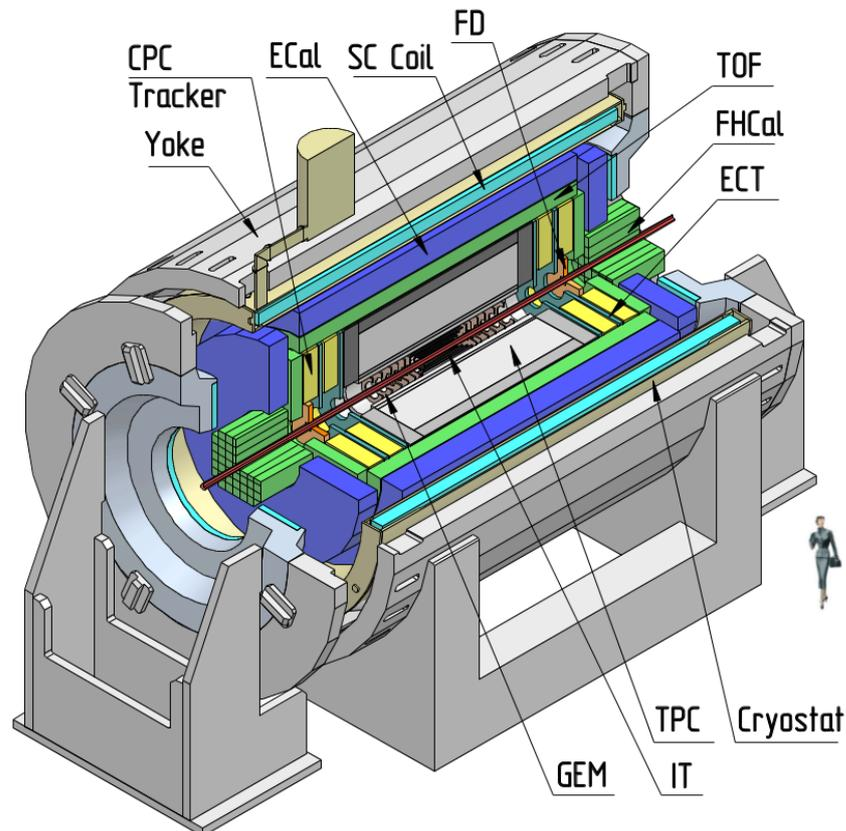
Figure 4: The Multi-Purpose Detector and the majors sub detectors and principal components appear. The MPD Central Detector (CD) is 6.6 meters in diameter and 9 meters long. **Image taken from <http://nica.jinr.ru/projects/mpd.php>**
