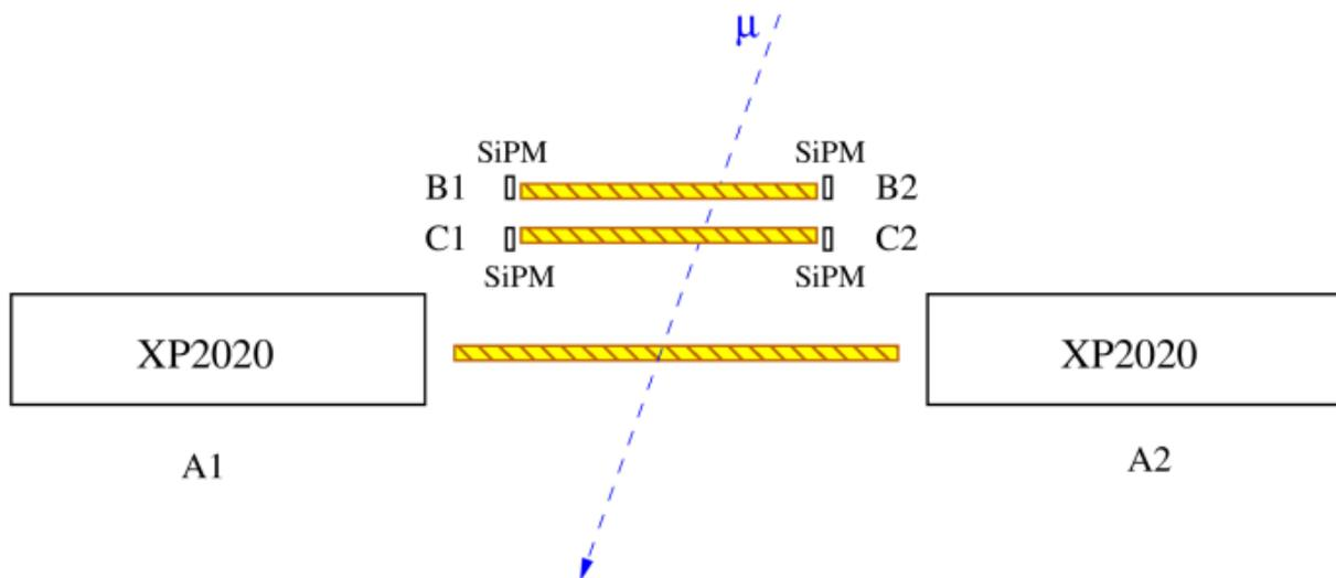
Figure 2: Schematic layout of the experimental setup.
