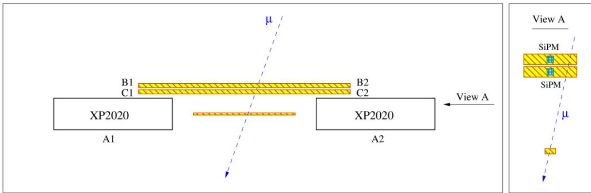
Figure 5: Placement of the counters in the cosmic stand efficiency measurement.
