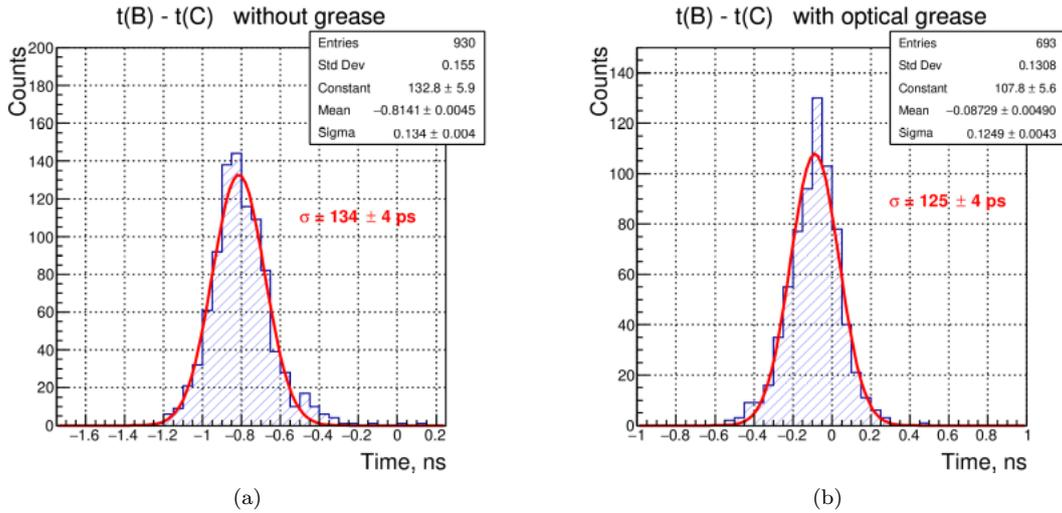
Figure 17: Time resolution between counters B and C.
