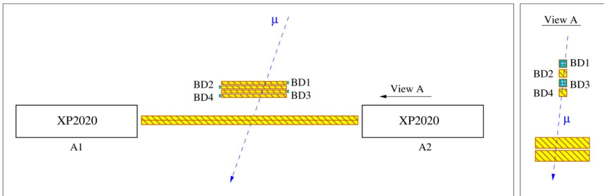
Figure 10: Placement of counters in the evaluation of Barrel Detector strips.
