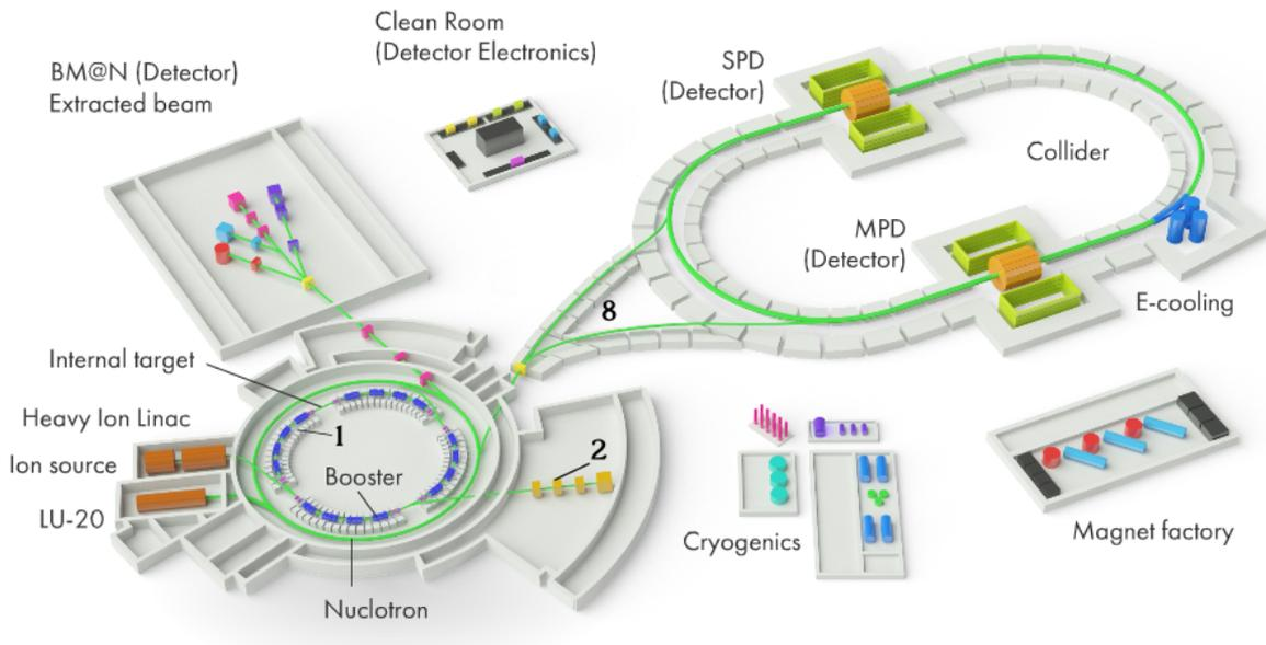
Figure 1: The principal components of the NICA accelerator complex appear. **Image taken from <http://nica.jinr.ru/complex.php>**
